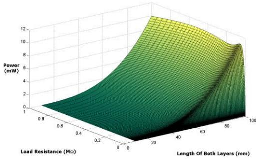
Fig. 5: Effect of beam length and load resistance on the harvester's power output while damping ratio remains constant.
