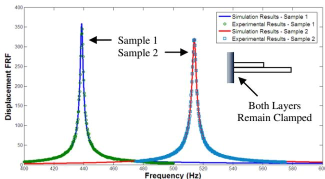
Fig. 9: Comparison between theoretical and experimental results for non-uniform samples.
