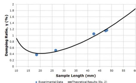
Fig. 1: The effect of sample length on the mechanical damping ratio.
