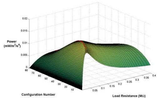
Fig. 7: Power dissipated across various load resistances for a range of harvester configurations with the same natural frequency.
