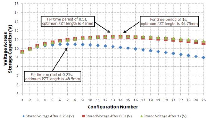
Fig. 8: Voltage across 500 nF capacitor against piezo length at three different time intervals. Substrate thickness used to maintain constant natural frequency.
