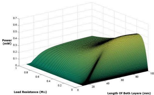
Fig. 6: Effect of beam length and load resistance on the harvester's power output while damping ratio is changing.
