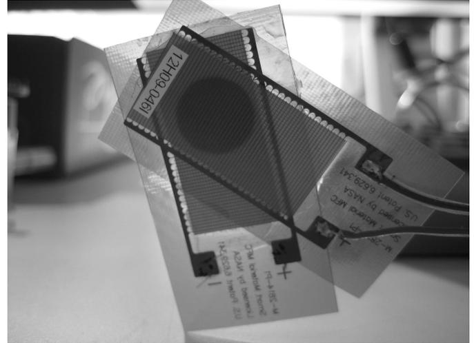
Figure 8: 100 mm FeSiB Metglass disc glued between 2 MFCs composites.
