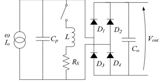
Fig. 6: Parallel SSHI with DC rectified output
