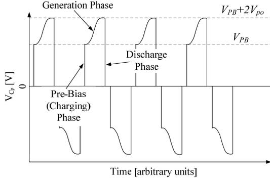
Fig. 3: Operational cycle showing charging and discharging of the piezoelectric capacitance  $C_p$
