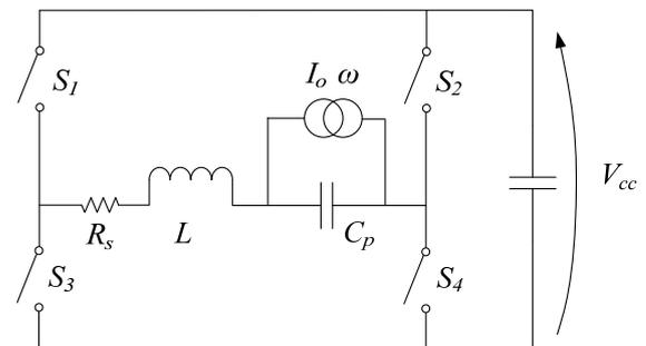
Fig. 2: Single-source pre-biasing circuit diagram
