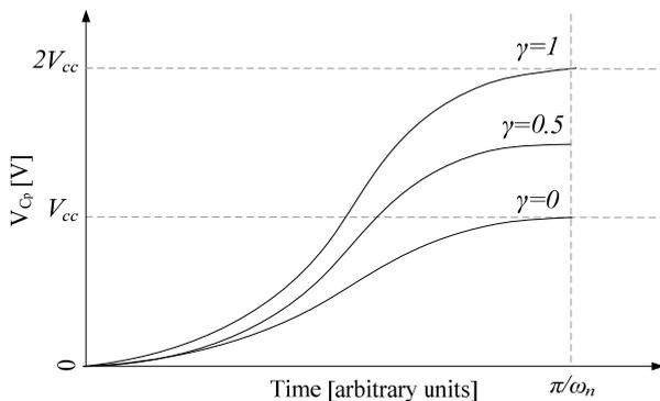
Fig. 4: Relationship between the loss coefficient  $\gamma$  and the final voltage after half a resonant charging cycle
