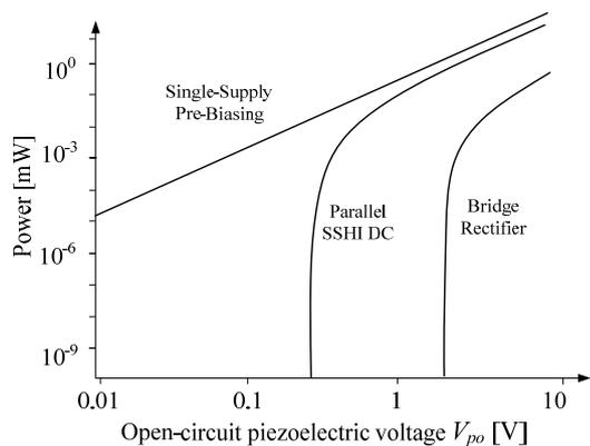
Fig. 9: Power comparison between circuits for low input excitation:  $V_D=1$ ;  $C_p=100$  nF;  $f_0=100$  Hz;  $Q=5$
