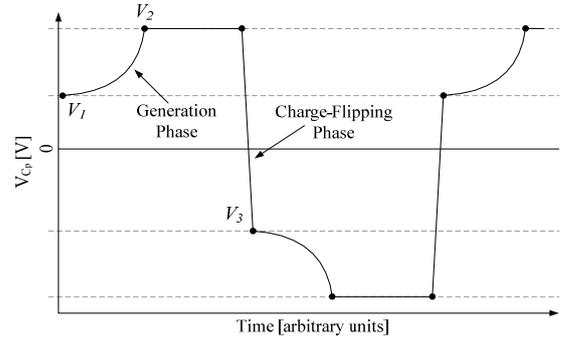
Fig. 7: Voltage waveform on  $C_p$  for Parallel SSHI DC
