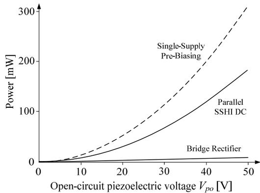
Fig. 8: Power comparison between circuits for:  $V_D=1$  V;  $C_p=100$  nF;  $f_0=100$  Hz;  $Q=5$
