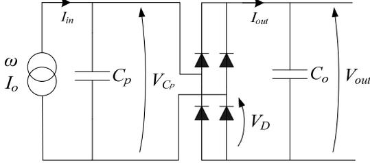
Fig. 5: Piezoelectric source with rectified DC load
