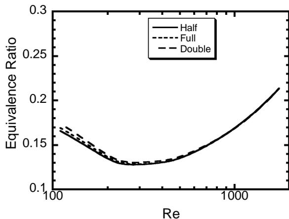
Fig. 3: The extinction limits of three different scale Swiss-roll combustors with constant  $\alpha$ ,  $R$ , and  $Da$ .
