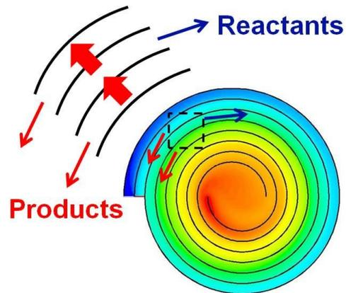
Fig. 4: Schematic diagram to show the heat loss from reactants to outer adjacent products.
