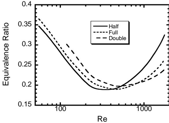
Fig. 2: The extinction limits of three different scale Swiss-roll combustors.
