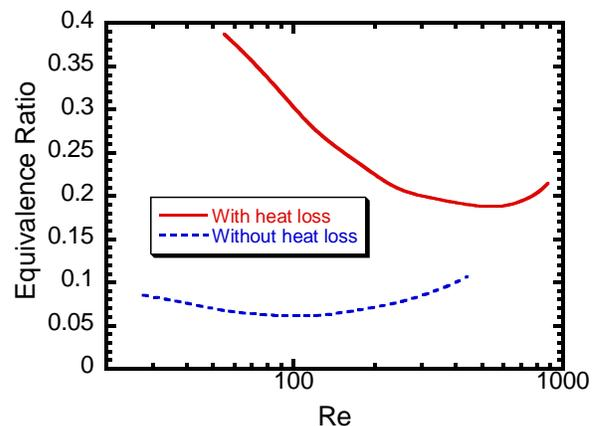
Fig. 5: Simulation results of the extinction limits with and without heat loss at low  $Re$ .
