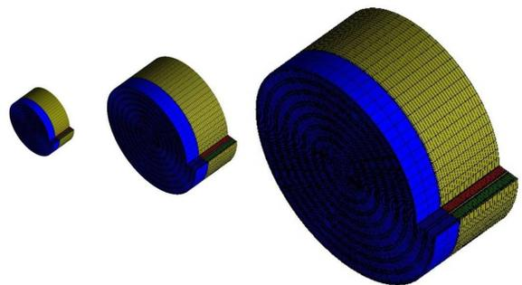
Fig. 1: Three different scale but geometrically identical 3.5-turn 3D numerical models of Swiss-roll combustors (Half, Full, and Double).
