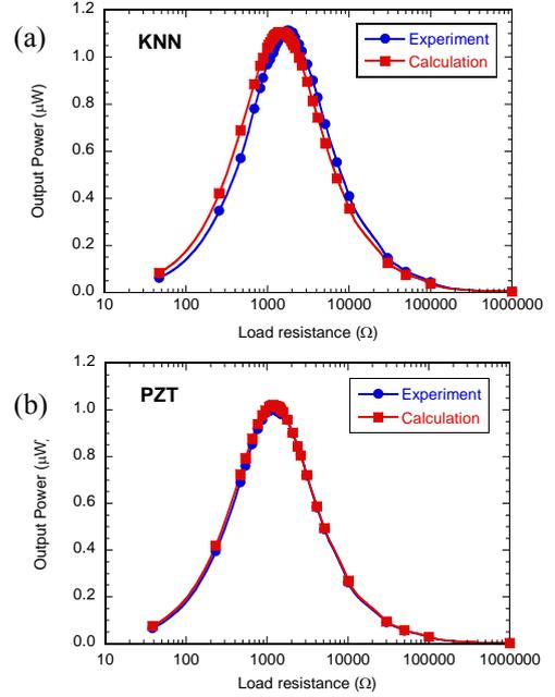
Fig. 6: Output power as a function of load resistance: (a) KNN/Si and (b) PZT/Si. Red and blue lines represent experimental and calculation, respectively
