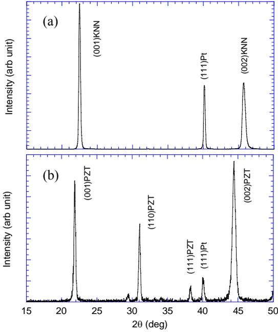
Fig. 1: XRD patterns: (a) KNN and (b) PZT thin films on Pt/Ti/Si substrates
