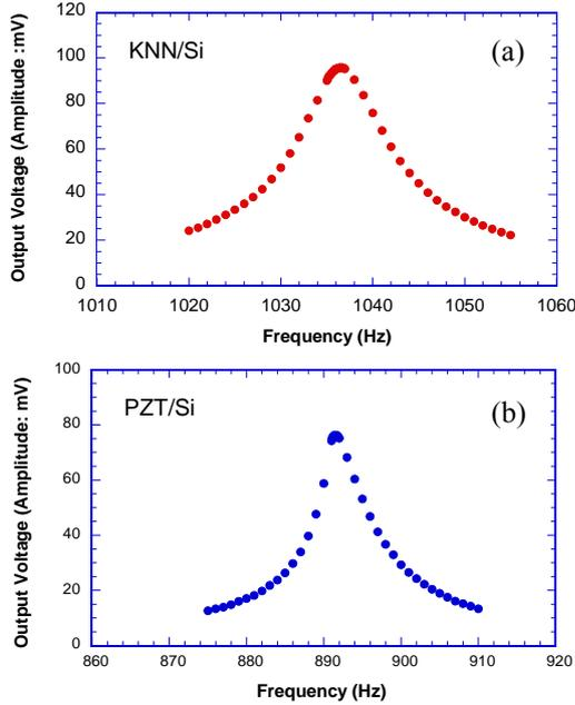
Fig. 5: Frequency response of output voltage: (a) KNN/Si and (b) PZT/Si energy harvesters
