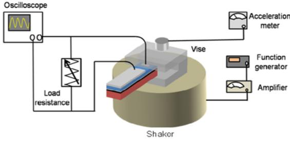
Fig. 4: Measurement setup of output power
