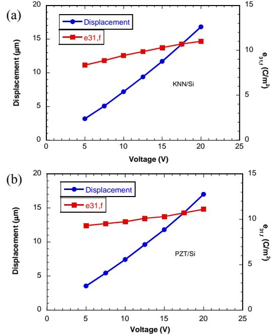
Fig. 3: Tip displacement of piezoelectric unimorph cantilevers and piezoelectric coefficient  $e_{31,f}$ : (a) KNN and (b) PZT thin films.
