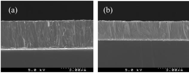
Fig. 2: Cross-sectional SEM images: (a) KNN and (b) PZT thin films
