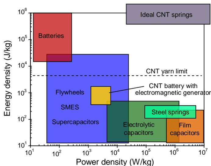
Fig. 8: Ragone plot comparing the energy density and power density of ideal CNT springs, the CNT-based battery with electromagnetic energy conversion, and conventional energy storage technologies [7, 8].
