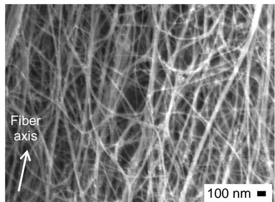
Fig 5: SEM images of yarn used as the spring for the CNT battery with an electromagnetic generator.
