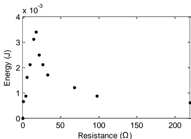
Fig. 7: Output electric energy as a function of output load resistance.
