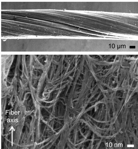
Fig 2: SEM images of the yarn used as the spring for the CNT battery with a piezoelectric generator.
