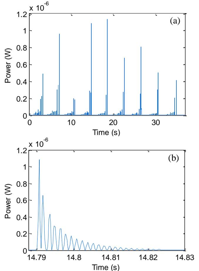
Fig. 3: Power output as a function of time for the CNT battery with a piezoelectric generator showing (a) the entire time of operation and (b) the oscillations in output power during the 40 ms following a collision between the cantilever beam and the gear.
