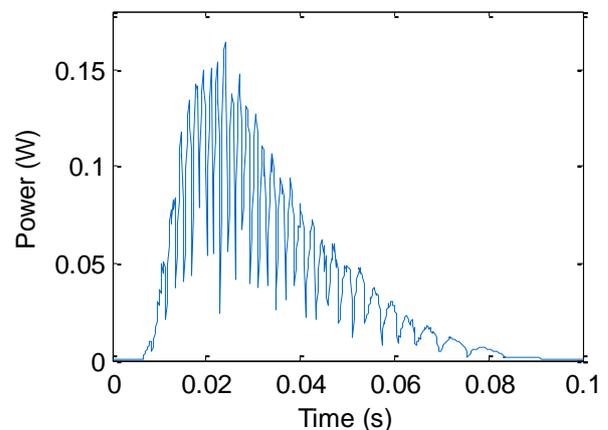
Fig. 6: Power output as a function of time for the battery with an electromagnetic generator.
