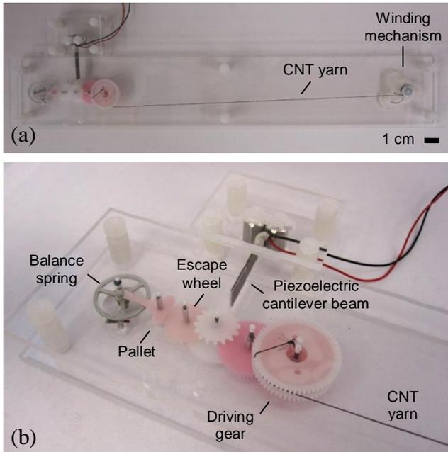
Fig. 1: CNT battery using a piezoelectric generator, showing (a) the entire system and (b) a close-up of the power regulation and energy conversion mechanism.
