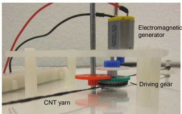
Fig 4: CNT battery using an electromagnetic generator.
