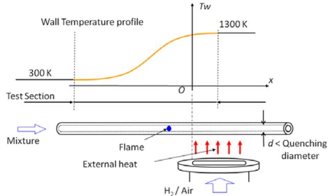
Fig. 2: Scheme of an apparatus consists of a meso-scale quartz channel and external heat source [7, 8]. Gas phase temperature profile is significantly governed by the prescribed temperature profile. Thus oxidation process in the channel is determined by the given temperature profile rather than the heat generation by itself particularly at low flow velocity.
