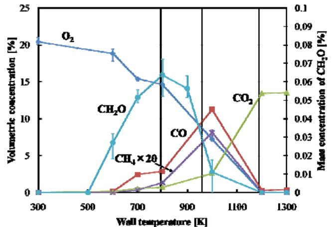
Fig. 9: Measured species concentration profiles of O<sub>2</sub>, CH<sub>2</sub>O, CH<sub>4</sub>, CO and CO<sub>2</sub> in multiple weak flames at inlet mixture flow velocity of 3.0 cm/s for n-heptane/air mixture ( $\phi = 1.0$ ). Three vertical lines are locations of three weak flames [10].
