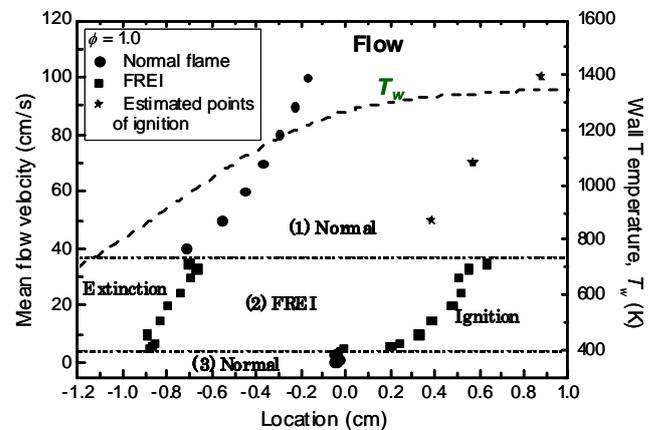
Fig. 4: Measured flame position and extinction and ignition points of FREI at various mean flow velocities for equivalence ratio,  $\phi = 1.0$ . Estimated ignition locations in upper normal flame regime are also indicated [7, 8].
