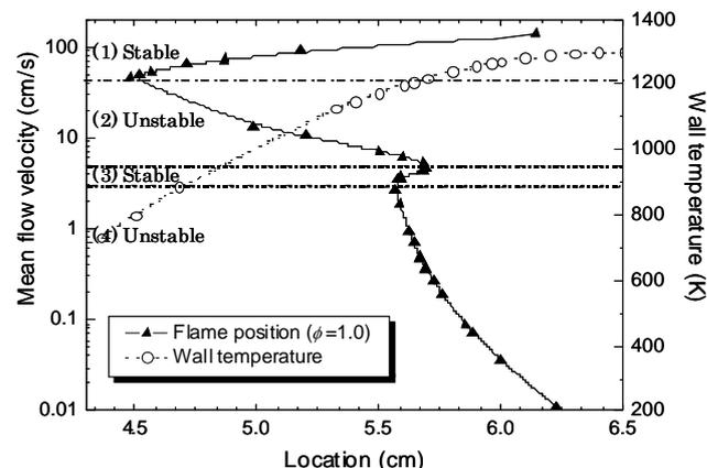
Fig. 6: Computational flame position as a function of inlet mixture flow velocity ( $\phi = 1.0$ ) [8]. Note that vertical axis for mean flow velocity is in log scale.
