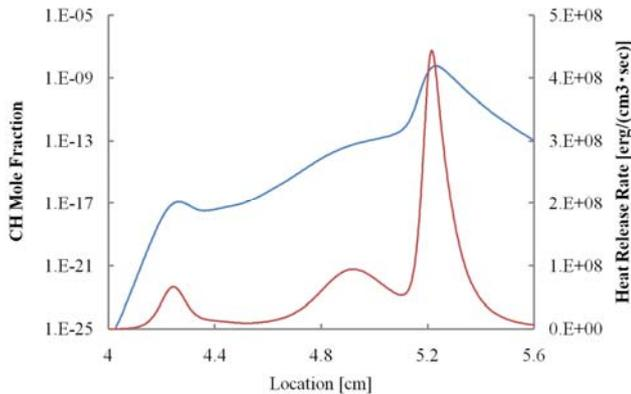
Fig. 8: Computational CH and heat release rate profiles for multiple weak flames observed at inlet mixture flow velocity of 3.0 cm/s for n-heptane/air mixture ( $\phi = 1.0$ ) [10].
