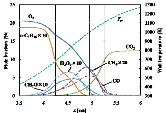
Fig. 10 Computational species concentration profiles of various chemical species in multiple weak flames at inlet mixture flow velocity of 3.0 cm/s for n-heptane/air mixture ( $\phi = 1.0$ ). Three vertical lines are locations of three heat release rate peaks [10].
