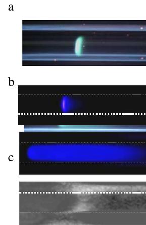
Fig. 3: Images of a) normal flame, b) Flames with repetitive extinction and ignition (FREI) and c) weak flames [7, 8].
