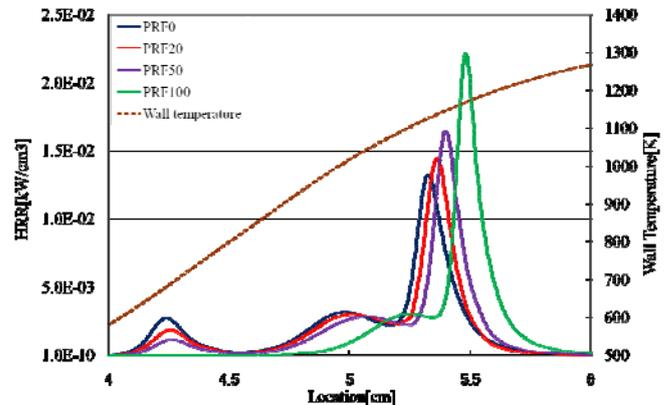
Fig. 12: Computational heat release rate profiles in weak flames at the inlet flow velocity of 12 mm/s for PRF/air mixture of RON 0, 20, 50 and 100 ( $\phi = 1.0$ ) [13].
