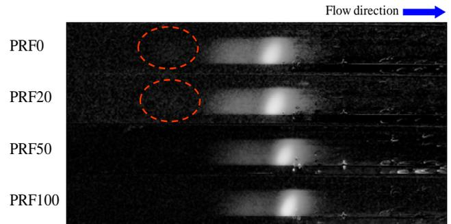
Fig. 11: Experimental weak flame images observed at the inlet mixture flow velocity of 12 mm/s for PRF/air mixture of RON 0, 20, 50 and 100 ( $\phi = 1.0$ ) [13].
