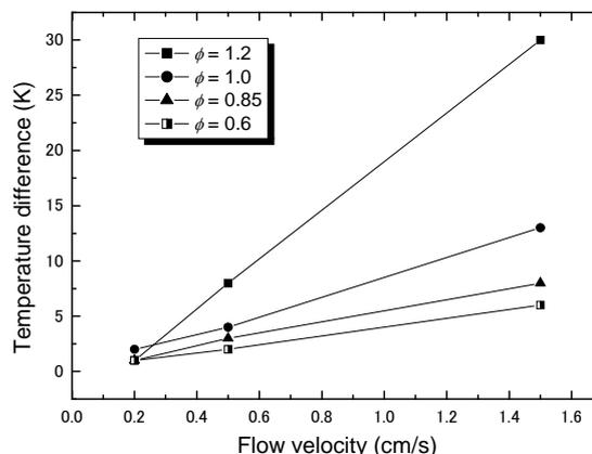
Fig. 5: Measured temperature difference between flame and the inner surface of the tube wall at the flame position ( $\phi = 0.6, 0.85, 1.0$  and  $1.2$ ) [8]. Temperature difference reduced to almost zero at lower flow velocity.
