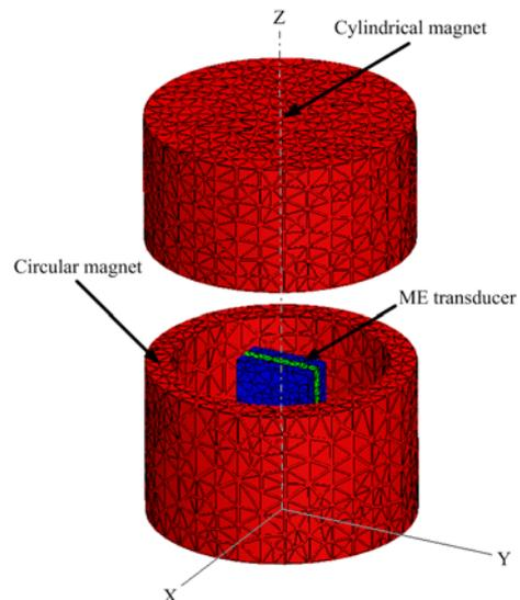
Fig. 4: Schematic diagram of the FEA simulation modal
