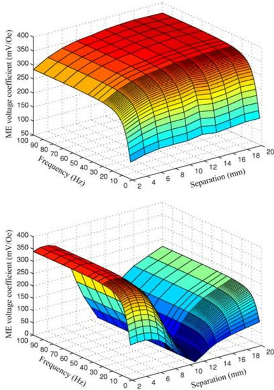
Fig.8: Measured ME voltage coefficient versus excitation frequency with different separation between the magnets. Top: repulsive mode, bottom: attractive mode.
