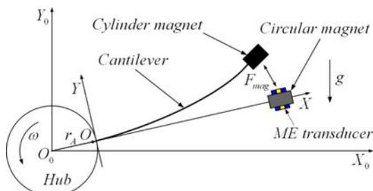
Fig.2: Structural model of the hub-beam system
