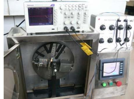
Fig.7: Experiment set-up for rotation energy harvesting
