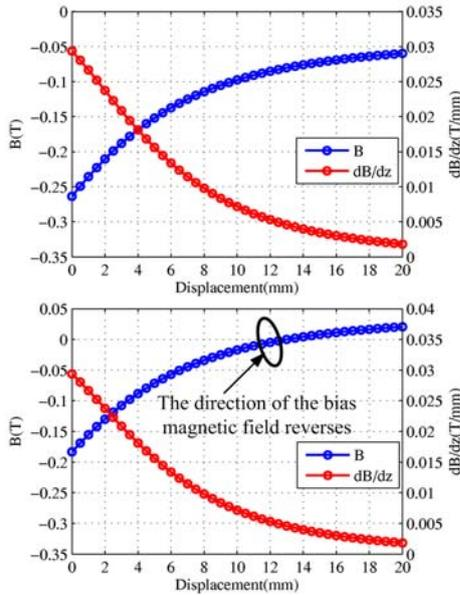
Fig. 5: Prediction of the magnitude and variation of  $B$  versus the separation between the magnets. Top: repulsive mode, bottom: attractive mode.
