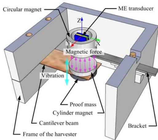
Fig.1: Schematic diagram of the proposed harvester.
