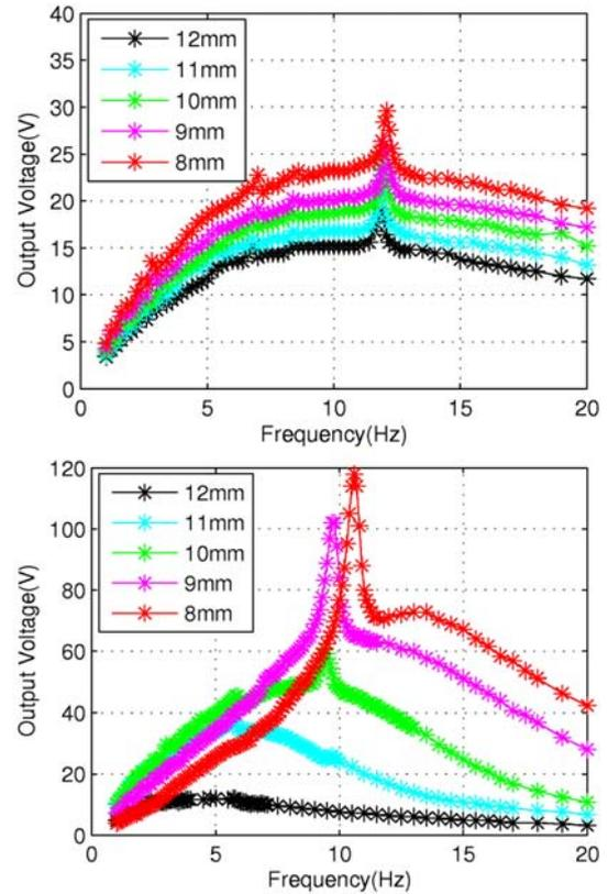
Fig.9: Open-circuit output voltage versus rotation frequency. Top: repulsive mode, bottom: attractive mode.
