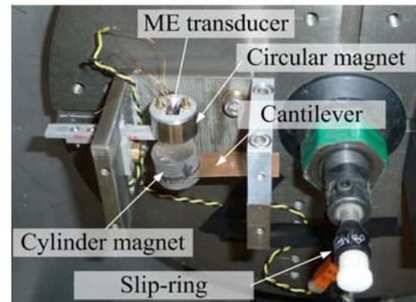
Fig. 3: Photograph of the proposed energy harvester
