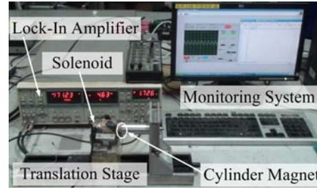
Fig.6: Experiment set-up for ME voltage coefficient
