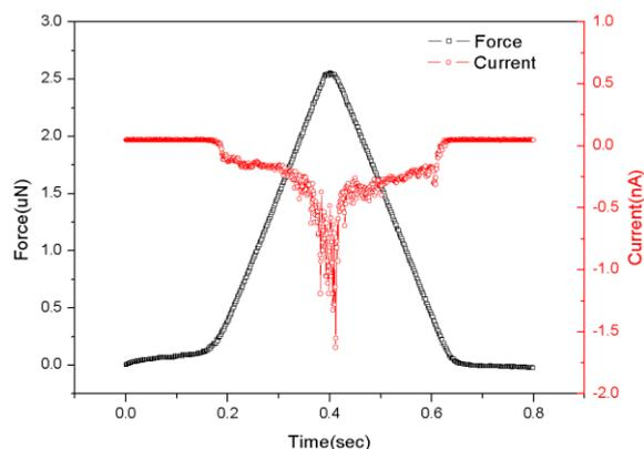
Fig. 5: Current measurement of GaN NW.
