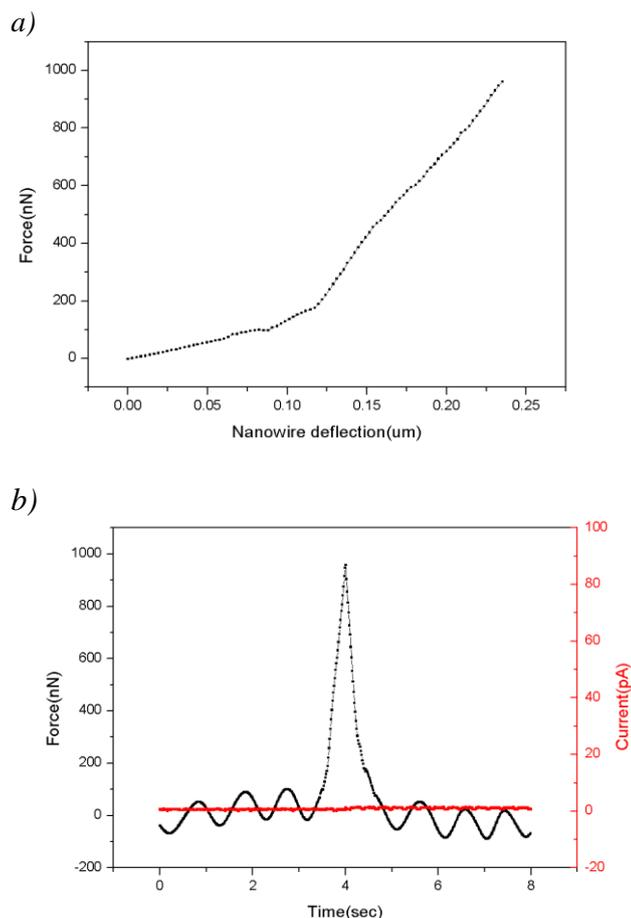
Fig. 4: (a) Deflection–force curve and (b) current generation during the bending of ZnO NW.
