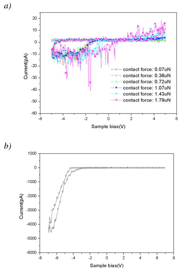
Fig. 3: a) I-V curves of ZnO NW measured at six stages of the bending process and b) I-V curve of ZnO NW entirely attached on gold electrode.
