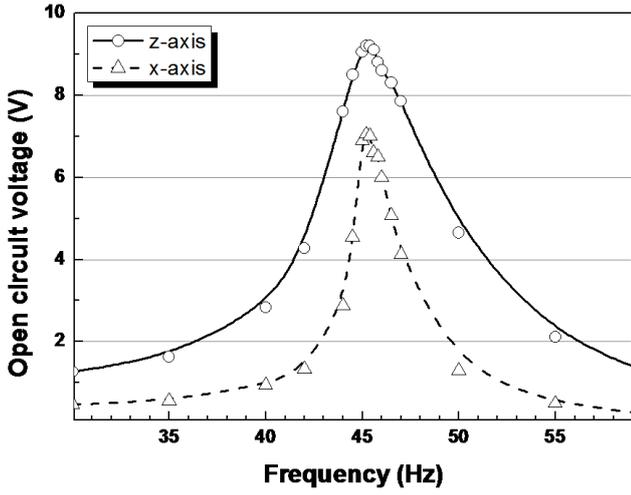
Fig. 4: The measured open circuit voltages of fabricated harvesting devices at induced vibration of  $1\text{m/s}^2$  of acceleration and frequencies ranged from 30 to 60 Hz.
