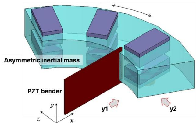
Fig. 1: Conceptual drawing of proposed piezoelectric power generator for two-dimensional vibration energy harvesting.
