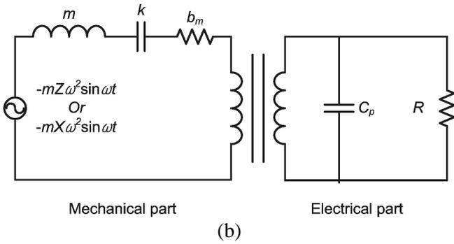
Fig. 2: Schematic drawing (a) and equivalent circuit representation (b) of proposed piezoelectric power generator.
