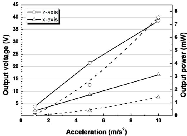
Fig. 6: The measured output load voltages (dotted line) and powers (solid line) of the fabricated harvesting device at its resonant frequency and various accelerations ranged from 1 to 10 m/s<sup>2</sup>.
