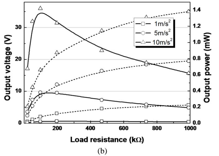
Fig. 5: The measured output load voltages (dotted line) and powers (solid line) of the fabricated harvesting device at various load resistances from z-axis (a) and x-axis (b) vibrations.
