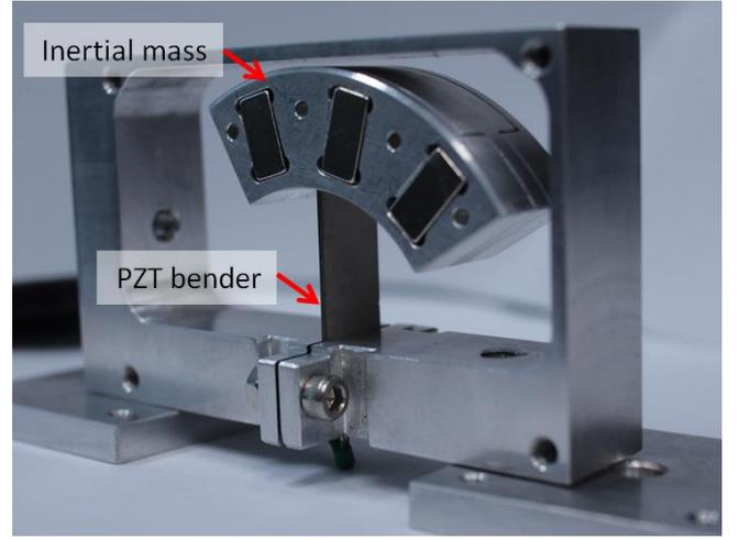
Fig. 3: Photomicrograph of fabricated device and fixture by using a bimorph PZT bender and an asymmetric aluminum inertial mass.
