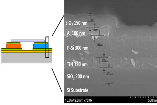
Fig. 4: SEM picture of the  $\mu$ -TEG.
