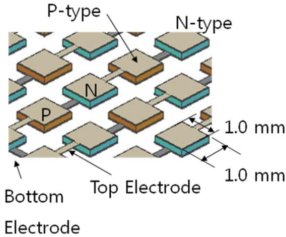
Fig. 2: Structure of the  $\mu$ -TEG.
