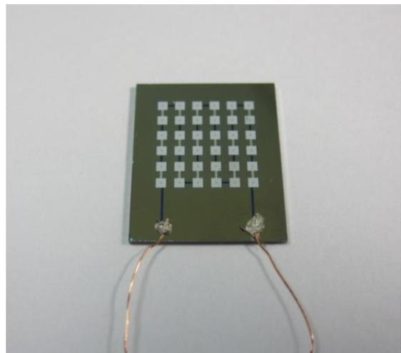
Fig. 1: Fabricated  $\mu$ -TEG.
