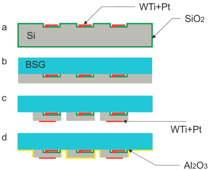
Fig. 3: Fabrication of the TG: (a) oxidized Si-wafer with metal parts of TCs, placed in grooves with contact windows at ends, (b) partial SiO<sub>2</sub> removal, anodic bonding and wafer thinning, (c) fabrication of contact pads and DRIE, (d) deposition of the isolation layer.
