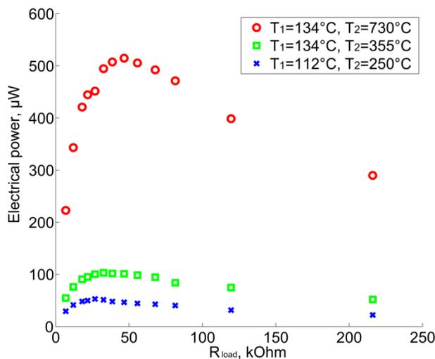
Fig. 7: Experimental points for power output versus consumer resistance at different temperature differences.
