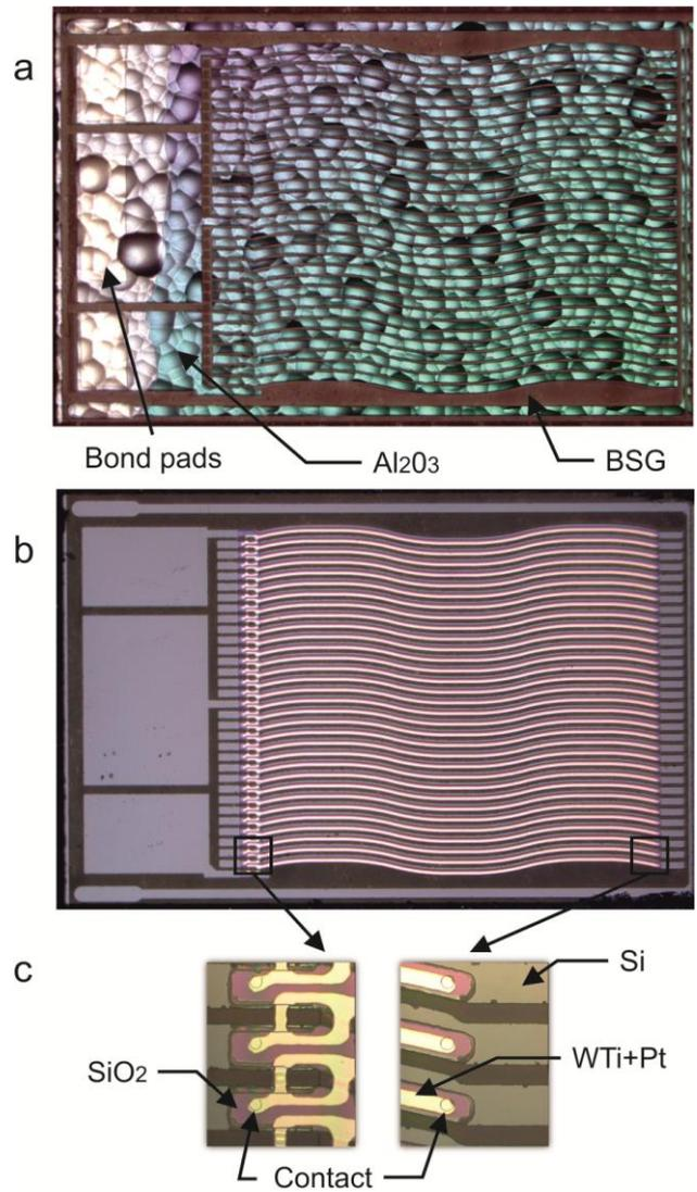
Fig. 2: Thermogenerator: (a) view from the structured side, (b) view through the transparent BSG-substrate, (c) blow-ups of the contact windows between Si and WTi+Pt.
