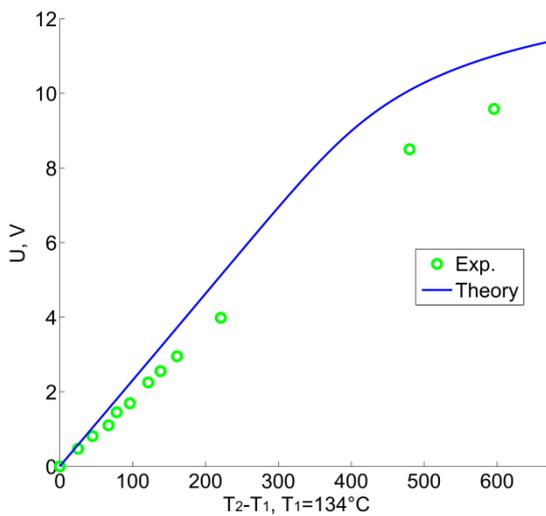
Fig. 6: Experimental points for open loop voltage versus the temperature difference in comparison with theoretical dependence.
