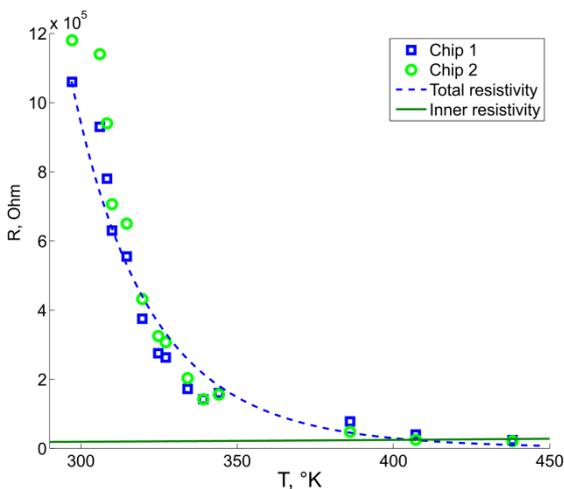
Fig. 4: Experimental temperature dependence of total resistivity of two TGs in comparison with theoretical values of the inner resistivity.
