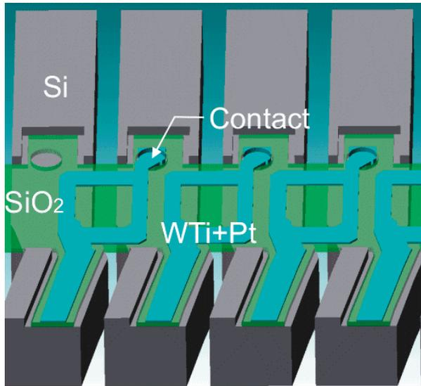
Fig. 1: Schematic of thermocouples.
