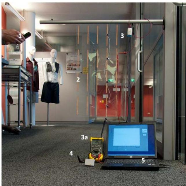
Fig. 7: Array consisting of four Yagi-Uda rectennas, connected in series, powering a wireless temperature sensor.
