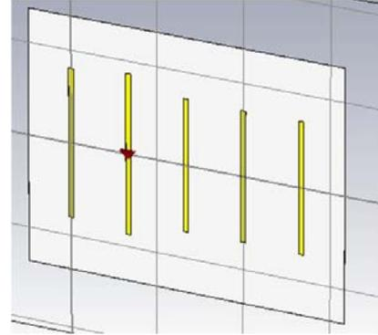
Fig. 4: Copper strip Yagi-Uda array antenna.
