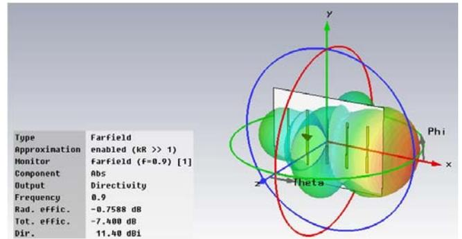
Fig. 5: Radiation pattern of copper strip Yagi-Uda array antenna.
