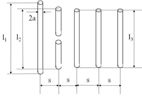
Fig. 3: Five elements, wire Yagi-Uda array antenna.
