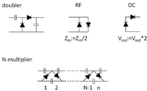
Fig. 1: Rectifier circuits. Top left: Voltage doubler. Top middle: RF equivalent of doubler. Top right: DC equivalent of doubler. Bottom: N-stage Cockroft-Walton voltage multiplier.
