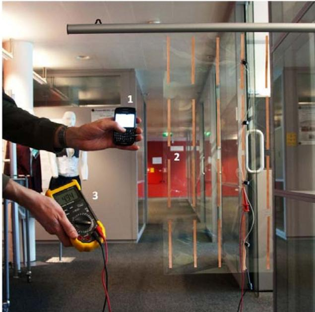
Fig. 6: Array consisting of four Yagi-Uda rectennas, connected in series.
