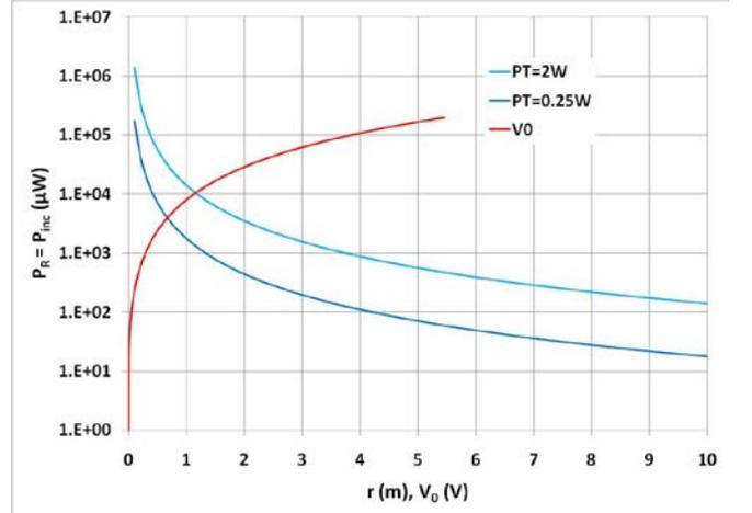
Fig. 2: Received power as a function of distance for two transmit power levels and rectifier output voltage as a function of incident power.
