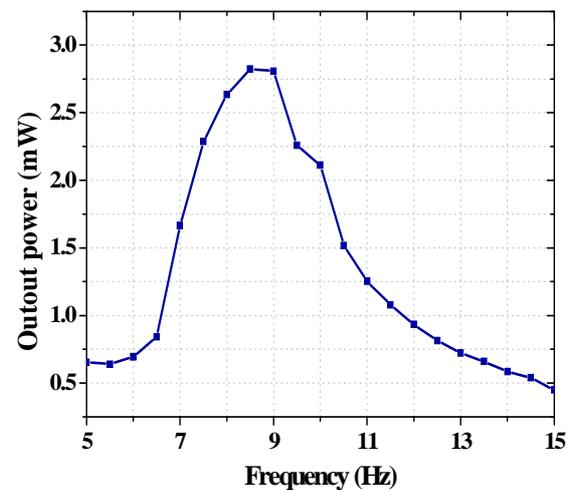
Fig. 6: Calculated output power of the fabricated harvester.
