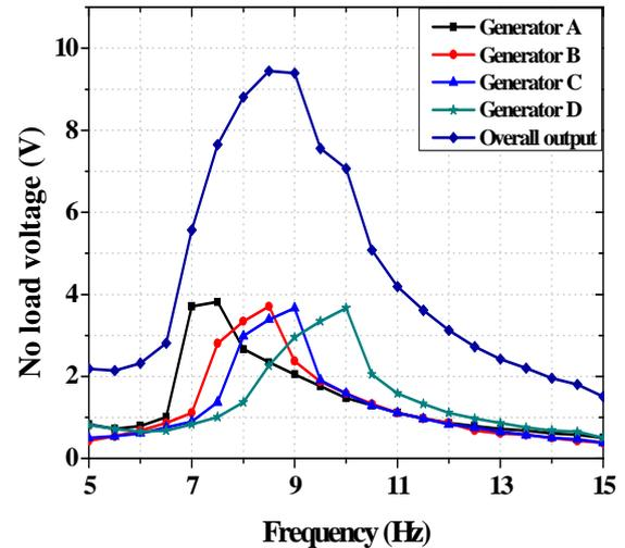
Fig. 5: Measured open circuit voltage for different input frequency.
