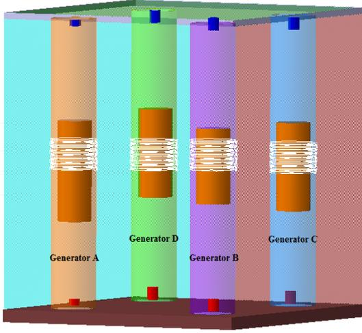
Fig. 2: Structure of the electromagnetic harvester array.
