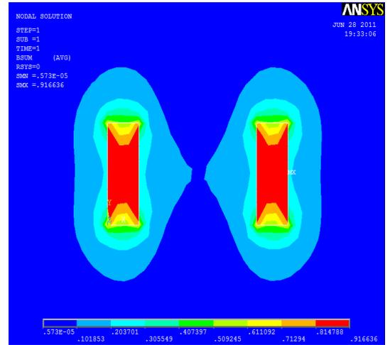
Fig. 3: Flux density distribution to find out the minimum spacing between individual generators.
