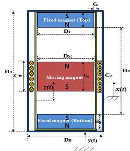
Fig. 1: Schematic diagram of the magnetic spring generator.
