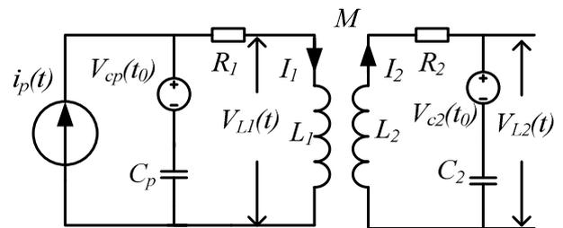
Fig. 5: Equivalent circuit when the switch is on
