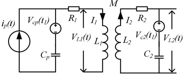
Fig. 6: Equivalent circuit when the switch is off
