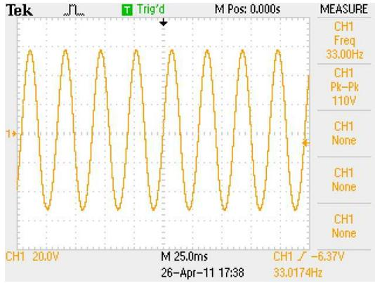
Fig. 1: The output of the harvester.
