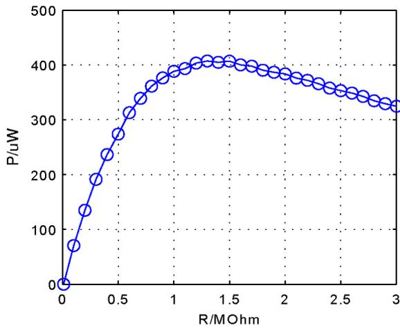
Fig. 2: Output power versus load resistance.
