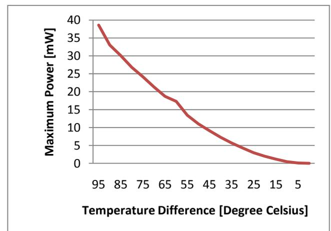
Fig. 5: Maximum power generation capability of the selected TE material in mW vs. degree Celsius
