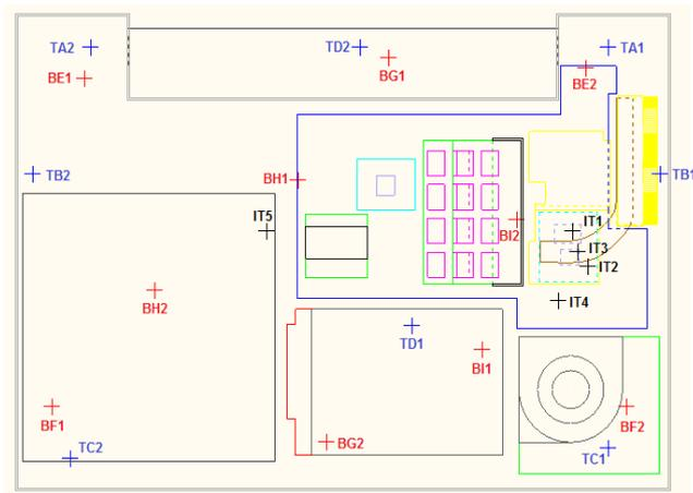
Fig. 2: Compact notebook temperature measurements (Prefix *T* stands for top layer, *B* for bottom layer and *I* for internal layers)
