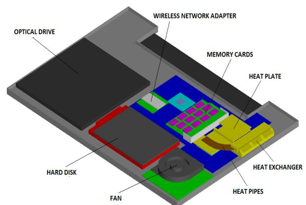
Fig. 1: Inner mechanical map of the target system. (Toshiba Portégé R705-P25)
