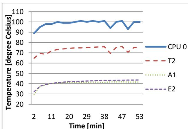
Fig. 3: Temperature variations of selected "hot spots" from inside and outside of the control system
