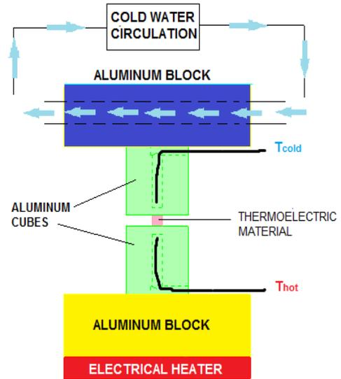
Fig. 4: TE module characterization setup
