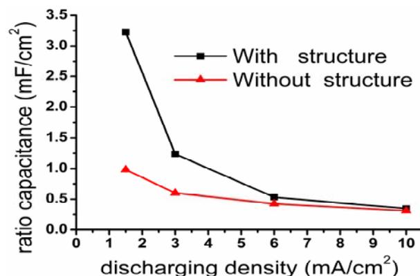
Fig. 5: electrode ratio capacitance comparison chart of with and without structure in different charging - discharging density
