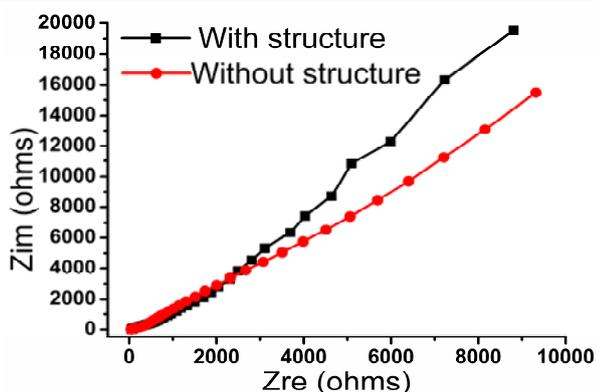
Fig. 3:  $MnO_2$  electrode AC impedance curve
