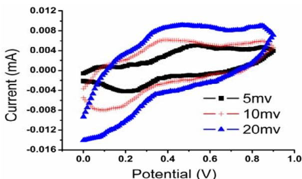
Fig. 2:  $MnO_2$  electrode cyclic voltammetry curve
