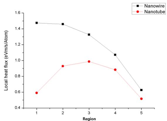
Figure 2. Local heat flux of NW (8,0) and NT (8,3) according to five divided regions. The values of the NW and NTs are normalized each other to have the identical temperature gradient.
