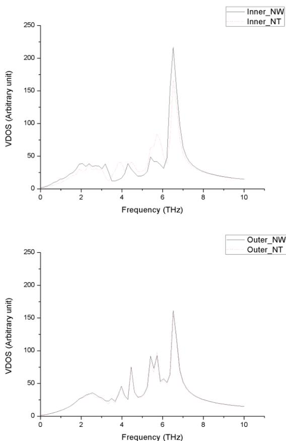
Figure 3. Local vibrational density of states on InAsNW and InAsNT at (a) Inner surface, (b) Outer surface.
