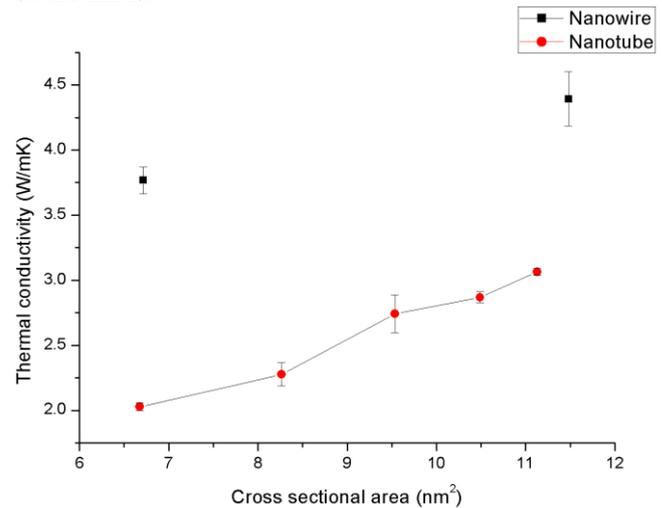
Figure 1. Thermal conductivities of two InAsNWs and five InAsNTs.
