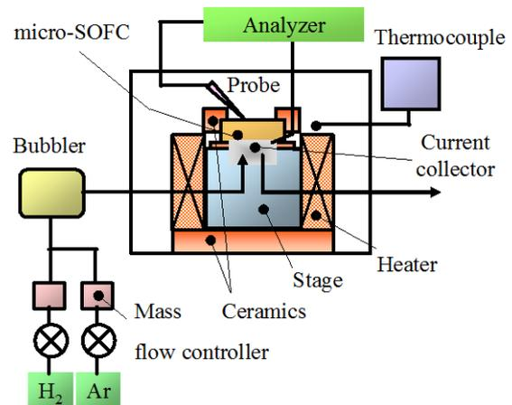
Figure 3 Schematic illustration of the testing apparatus.
