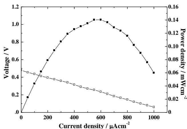
Figure 6 I-V and I-W characteristics of the micro-SOFC with the internal micro heater.
