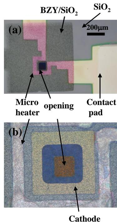
Figure 4 Optical images of the micro-SOFC with the internal micro heater. (a) : Overview from cathode side. (b) : Close-up
