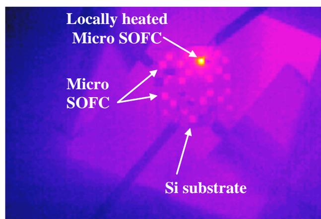
Figure 5 Image of an infrared camera in the power generation test.
