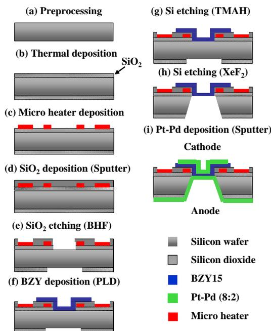
Figure 2 Diagrams of the fabrication process of the micro-SOFCs. BHF: Buffered hydrofluoric acid; TMAH : Tetramethylammonium hydroxide
