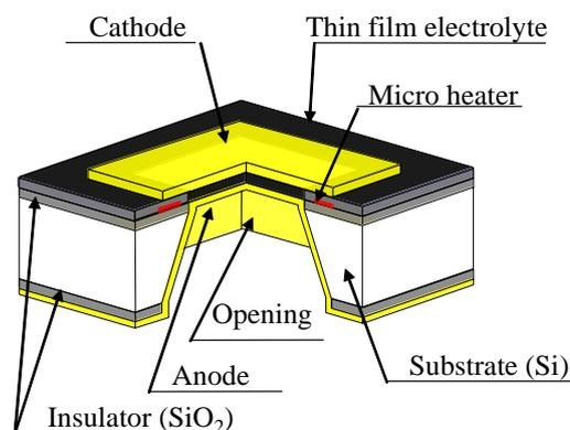
Figure 1 Schematic illustration of the micro-solid oxide fuel cell design with an internal micro heater.
