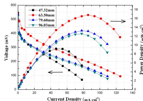
Fig. 5 The effect of the channel lengths of the anode flow field on the  $\mu\text{DMFC}$  performance.
