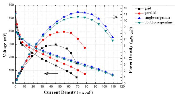
Fig. 3 The effect of the anode flow field structures on the  $\mu\text{DMFC}$  performance.
