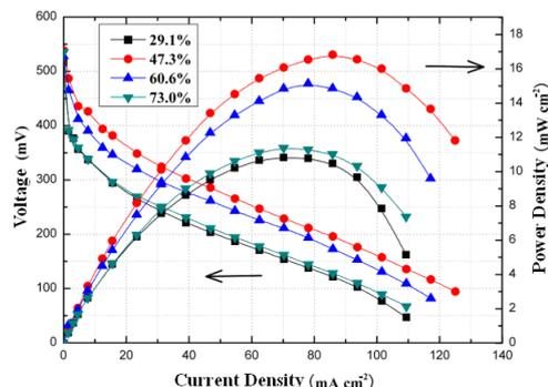
Fig.4 The effect of the opening ratios of the anode flow field on the  $\mu\text{DMFC}$  performance.
