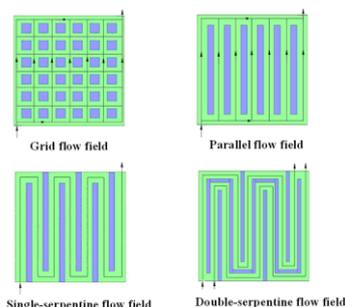
Fig. 1 Design of the anode flow fields
