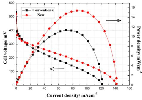
Fig. 6 Performance comparisons of the self-breathing  $\mu$ DMFCs with the conventional and new single serpentine flow fields
