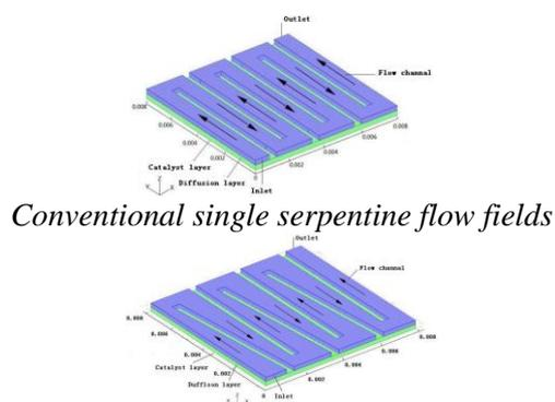
Fig. 2 Design of the anode flow fields
