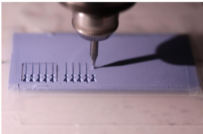
Fig. 6: Micro milling during preparation of the capillary fuel tubes.
