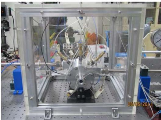
Figure 3. Assembled UMGH compressor performance evaluation equipment on the test bed.
