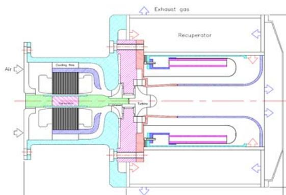
Figure 1 Schematics of the ultra-micro gas turbine
