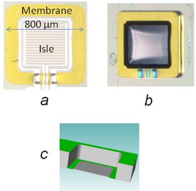
Fig. 3: Unsealed TG's prototype: (a) photo of the front side, (b) photo of the back side, (c) the cross section of the structure.
