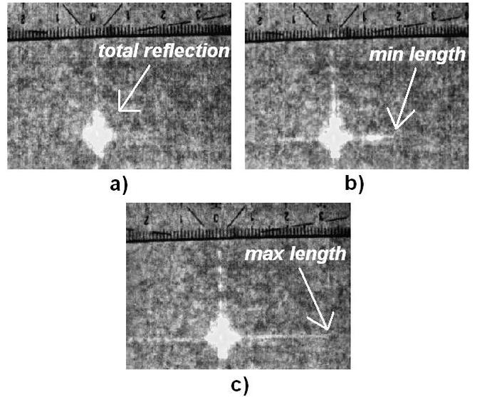
Fig. 6. Projections of the reflected laser beam: (a) inert membrane, (b) minimal deflection, (c) maximal deflection.
