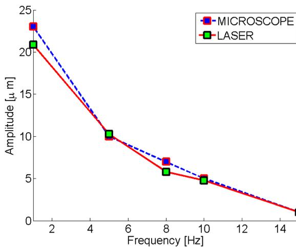
Fig. 7. Experimental points for the vibration amplitude versus its frequency.
