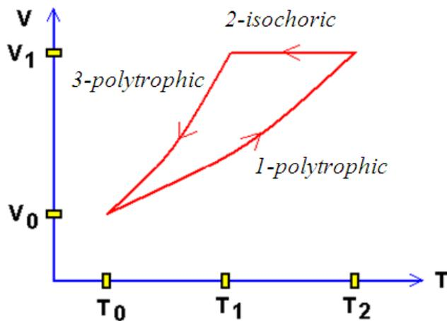
Fig. 2: Working cycle of the heat engine.
