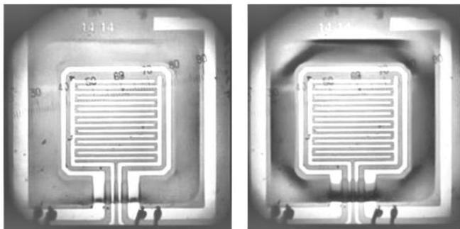
Fig.8. Vibrating membrane in low and high positions. The membrane deflection is 22μm.
