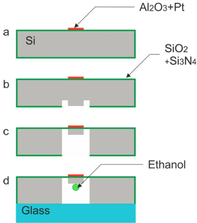
Fig. 4: Fabrication of the TG's prototype: (a) oxidized Si-wafer with silicon nitride and the heater, (b) isle's definition on the back side, (c) DRIE-fabrication of isle, (d) deposition of fluid's drop and chamber sealing.
