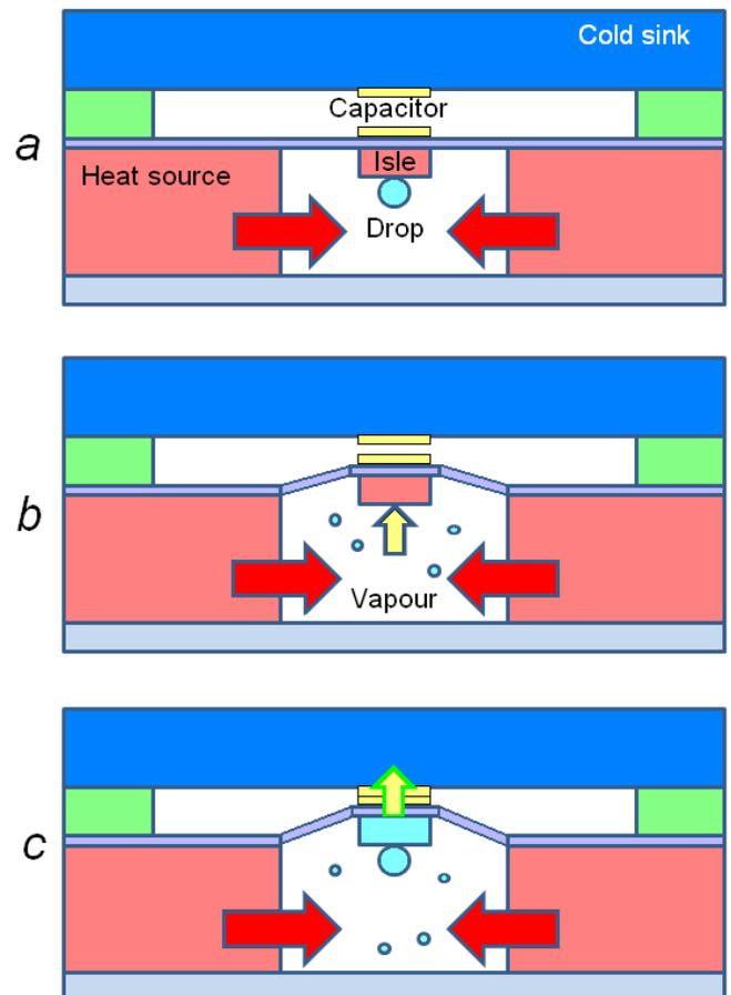
*Fig. 1: TG's design and working principle: (a) the working liquid-gas mixture is heated up, (b) the rising pressure pushes up the isle, (c) the isle is cooled down by the cold sink, the working gas condenses.*
