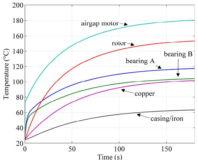
Fig. 4: Temperature increase at various locations within the system.
