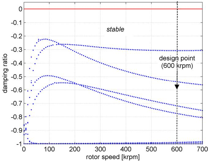
Fig. 2: Damping ratio as a function of the rotational speed.
