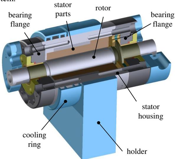
Fig. 5: CAD cut-away view of the experimental system.
