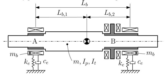
Fig. 1: Bearing configuration and rotordynamic model.
