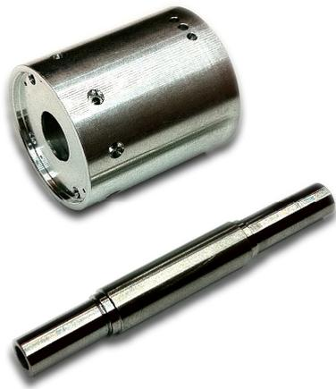
Fig. 6: Stator cooling housing and rotor (without bearing parts) of the experimental setup.
