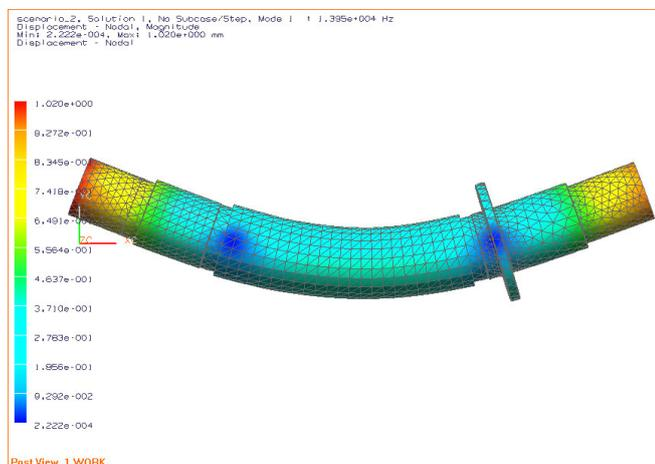
Fig. 3: First bending mode of the rotor at 13.95 kHz.
