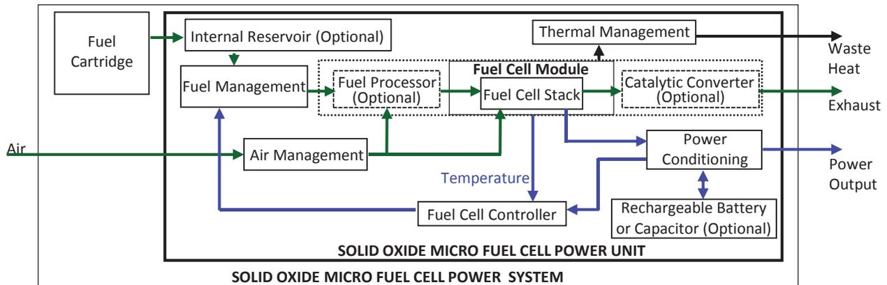
Figure 3: Butane Fuel Cell System block diagram.[9]
