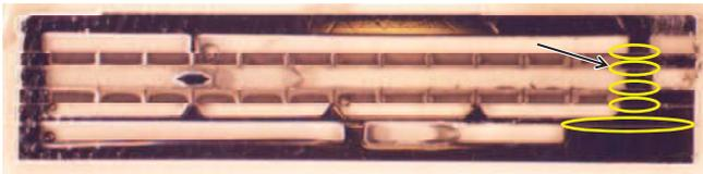
Figure 7: Cross section of an assembled silicon die stack using Lilliputian's glass seal.
