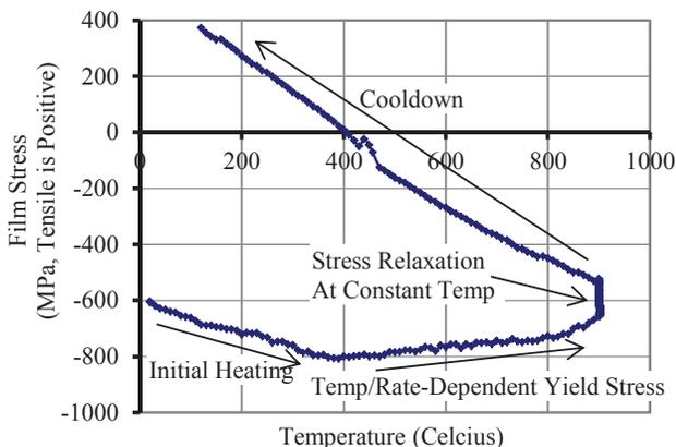
Figure 8: Stress vs. Temperature during the first thermal cycle of an example YSZ film. Thickness 2  $\mu\text{m}$ , heating and cooling rates of 6 °C/min, dwell time of 3 hrs.
