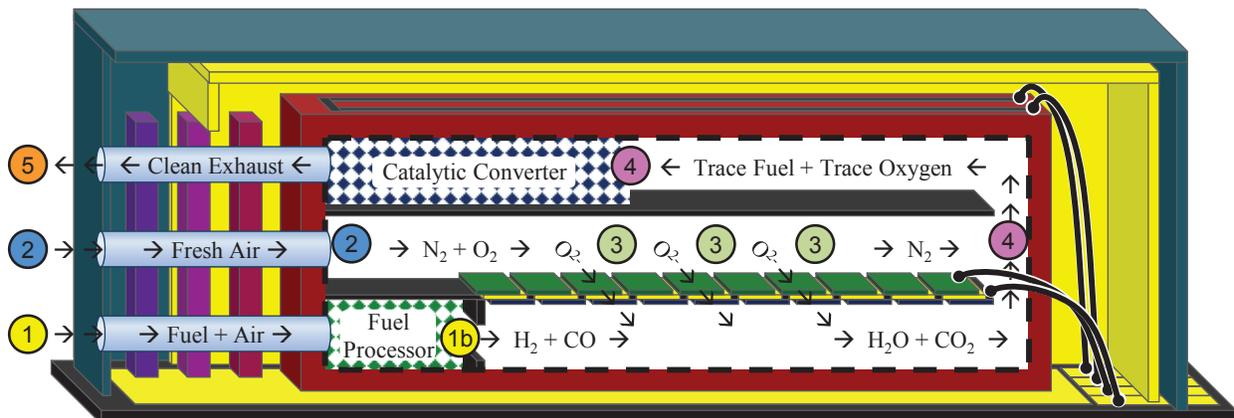
Figure 4: Schematic of Lilliputian's Generator Chip
