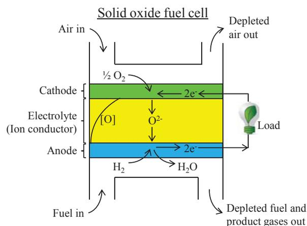
Figure 2: SOFC operating principle
