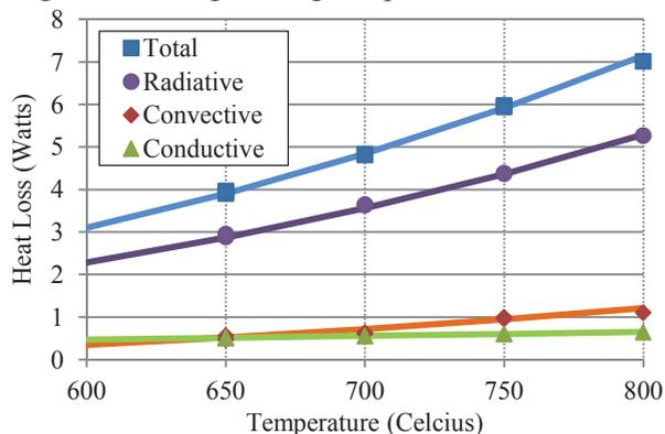
Figure 6: Extreme insulation measured on a representative Generator Chip.
