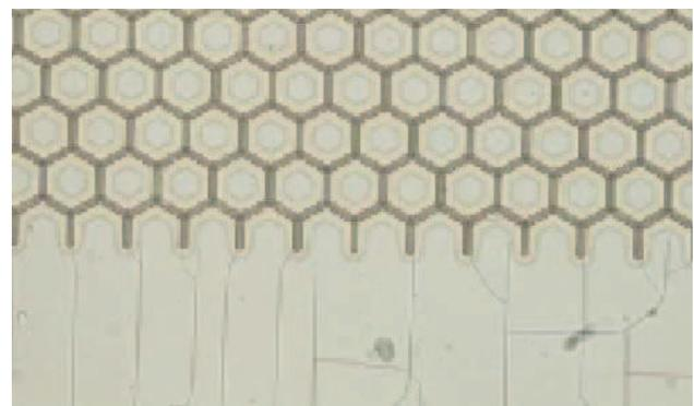
Figure 9: Simplified process flow for the Pre-Cracked fuel cell and a micrograph of the edge of a Pre-Cracked region
