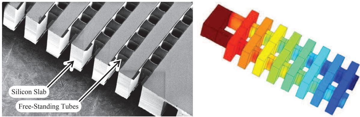
Figure 5: (Left) Electron-micrograph of MEMS Tubes, (Right) Modeling of heat recovery characteristics.
