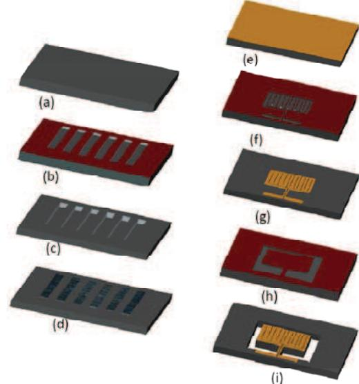
Fig. 3: Fabrication process of the multi-pole electrodynamic energy harvester.
