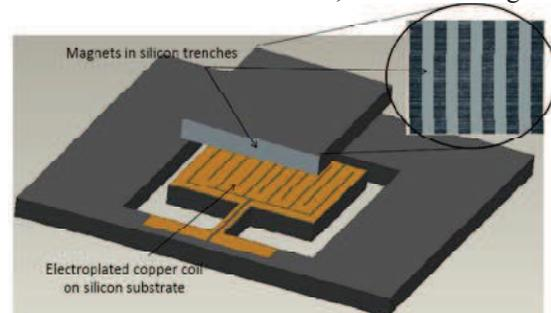
Fig. 1: Schematic of electrodynamic vibrational energy harvester with multi-pole architecture.
