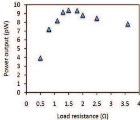
Fig. 7: Power output versus load resistance of the energy harvester at 1 g acceleration.
