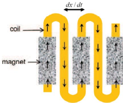
Fig. 2: Top view of magnet/coil arrangement for multi-pole architecture. Arrows represent the flow of current in the coil. Note that the magnets are magnetized in out of plane.
