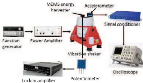
Fig. 5: Experimental setup of the electrodynamic energy harvester.
