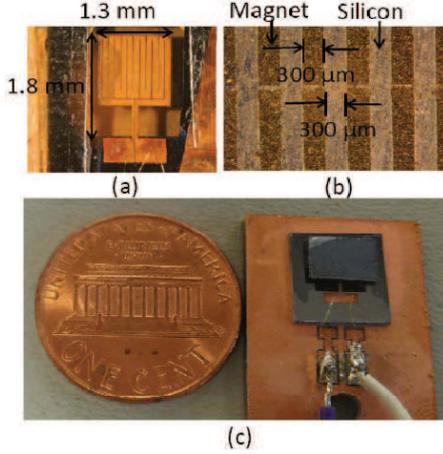
Fig. 4: (a) Silicon cantilever beam with serpentine electroplated copper coil on top, (b) Bonded-powder NdFeB magnets in silicon trenches, (c) Assembled device on a PCB board.
