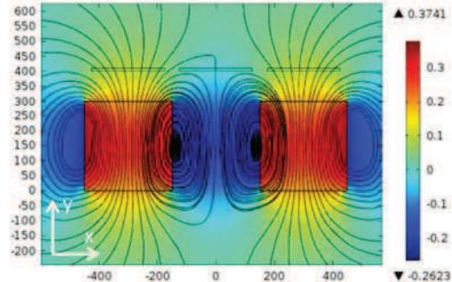
Fig. 6: Simulation of magnetic flux density ( $B$ -field) in the  $y$ -direction from the magnetic arrays.
