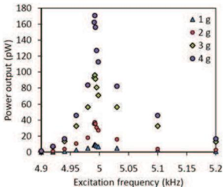
Fig. 8: Power output versus excitation frequency of the energy harvester at 1 g, 2 g, 3 g, and 4 g acceleration.
