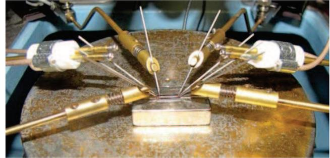
Fig. 3: Picture of the device measurement setup.
