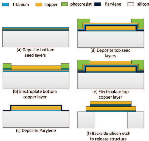
Fig. 2: Fabrication process of the micro-ET.
