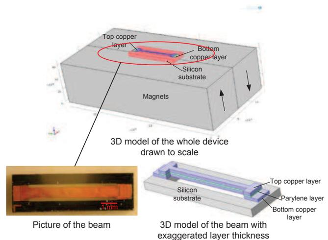
Fig. 1: Schematic and picture of the ET.
