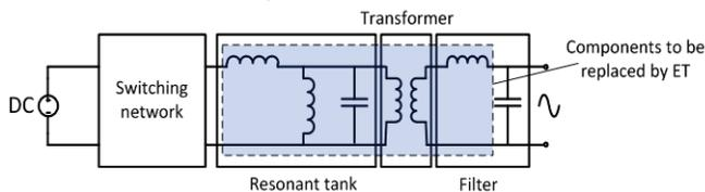
Fig. 6: LLC-PRC resonant inverter using ET.
