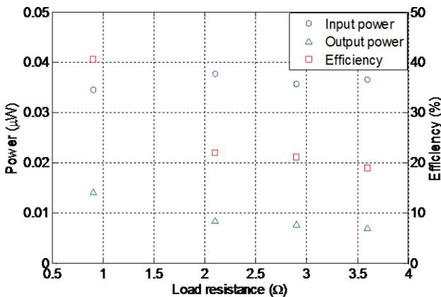
Fig. 5: ET input/output power and efficiency vs. load resistance.
