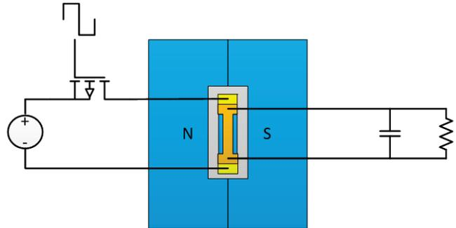
Fig. 7: Illustration of the ET-based inverter.
