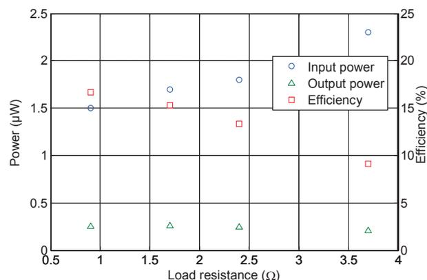
Fig. 9: Input/output power and efficiency of the resonant inverter.
