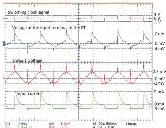
Fig. 8: Waveforms of the resonant inverter.
