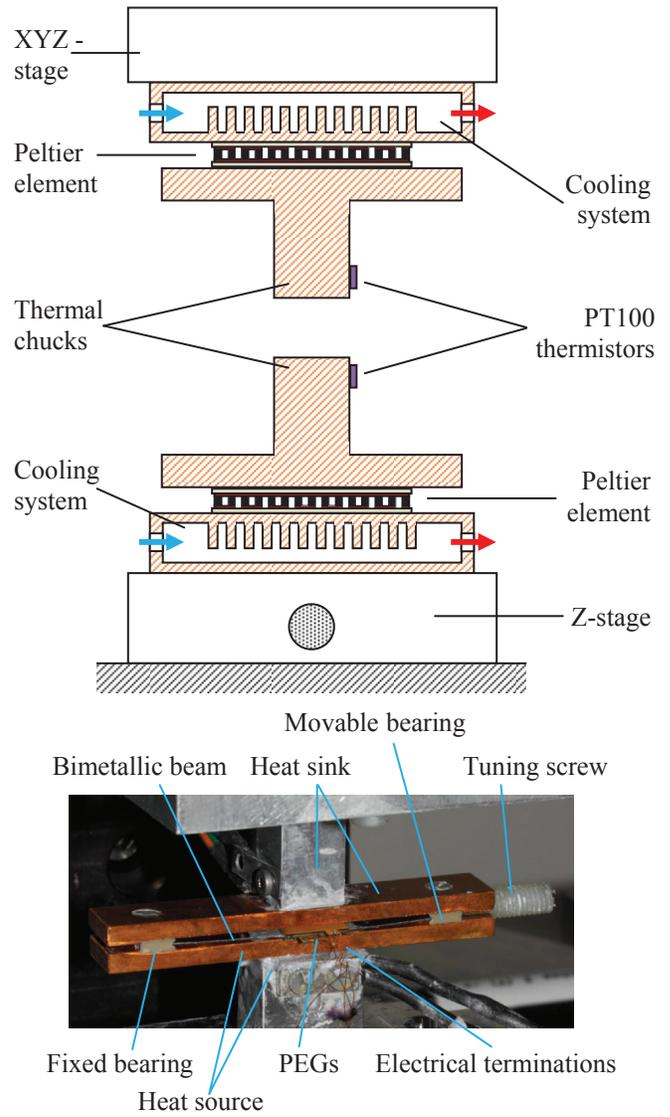
Figure 4: Schematic drawing of the test setup used to characterize the harvester (top) and photograph of a pyroelectric harvester in the test setup. Both the thermal chucks are capable of functioning as either a heat source (hot side) or sink (cold side). In this work the upper chuck is used as the hot side and the lower one as the cold side. This reduces the influence of convection to a great extent.
