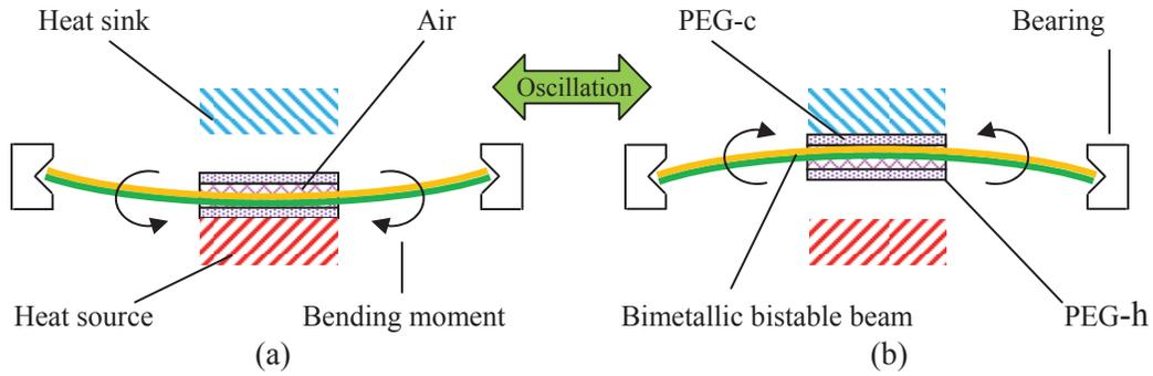
Figure 1: Schematic of the operation principle of the pyroelectric harvester, showing the PEGs and beam in contact with the (a) heat source and (b) sink . PEG-c and PEG-h indicate the PEG near to the cold and hot sides respectively.
