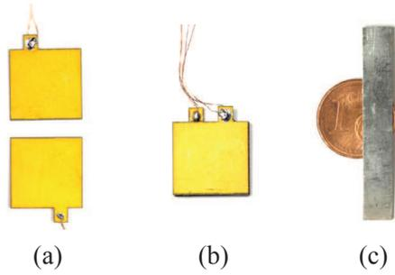
Figure 3: a) Fabricated PEGs with soldered wires b) PEG assembly and c) bimetallic strip. The PEGs are kept one over another, with a 300  $\mu\text{m}$  spacer in-between. Thereafter, glue is applied to the top and bottom edges. The spacer is removed once the glue has set. Subsequently, the beam is inserted into the gap between the PEGs.
