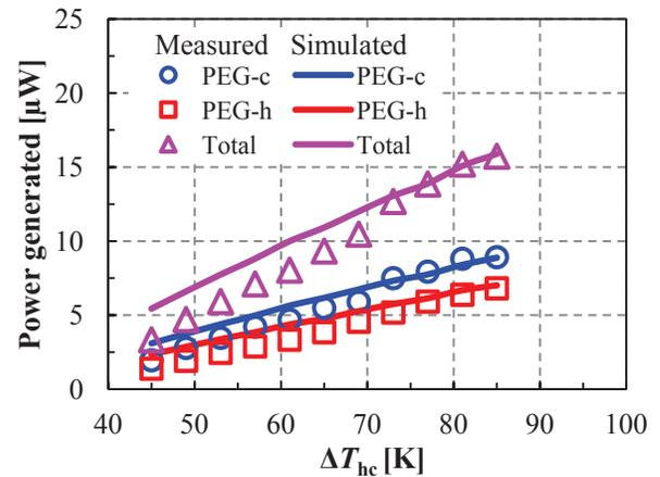
Figure 7: Dependency of the power generated by each PEG and of the total power on  $\Delta T_{hc}$ .
