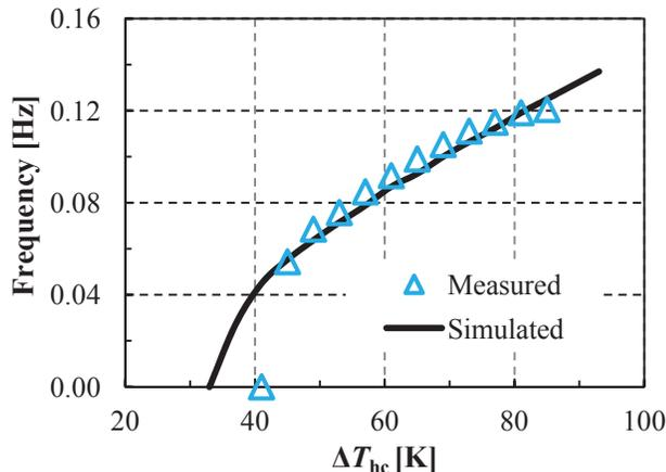
Figure 6: Variation of the operational frequency  $f$  with the temperature difference between the heat source and sink ( $\Delta T_{hc}$ ).
