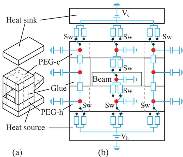
Figure 2: Electrical network elements of the PEGs with inserted bimetallic beam, with thermal resistances, capacitances and switches representing the operation and thermal characteristics of the harvester.
