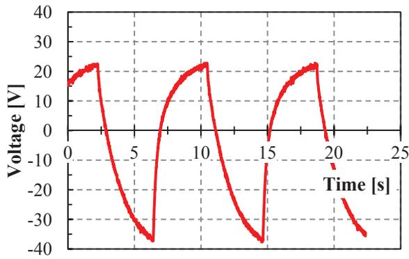
Figure 5: Recorded open circuit voltage waveform across PEG-c for temperatures of 108 °C and 23 °C at the hot and cold side, respectively.
