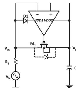
Figure 4. Schematic of the primary rectifier
