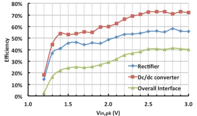
Figure 8. Circuit efficiency at different input voltage amplitudes ( $f=20$  Hz) when charging a 3.7 V battery
