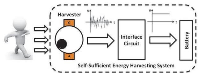
Figure 1. Block diagram of the self-sufficient energy harvesting system
