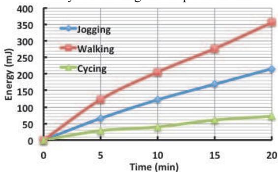
Figure 9. Energy delivered to the battery for the system mounted on the human ankle
