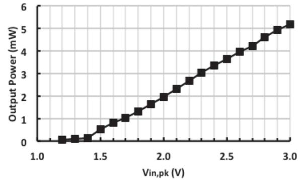
Figure 6. Power delivered to 3.7 V battery at different input voltage amplitudes ( $f=20$  Hz)
