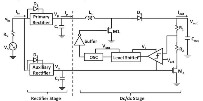
Figure 3. Block diagram of the interface circuit
