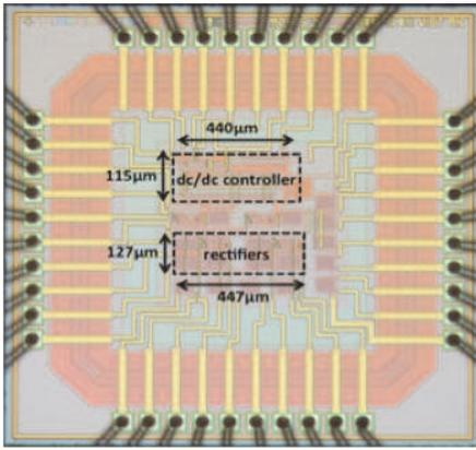
Figure 5. Micrograph of the interface circuit chip
