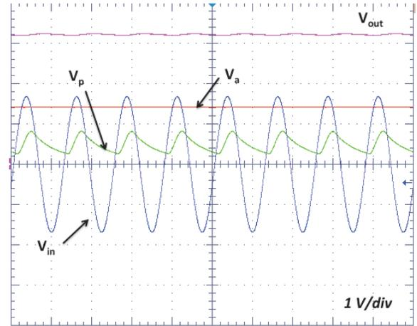
Figure 7. Measurement result at 7.5 k $\Omega$  load when input is a 20 Hz, 1.7 V amplitude sine wave
