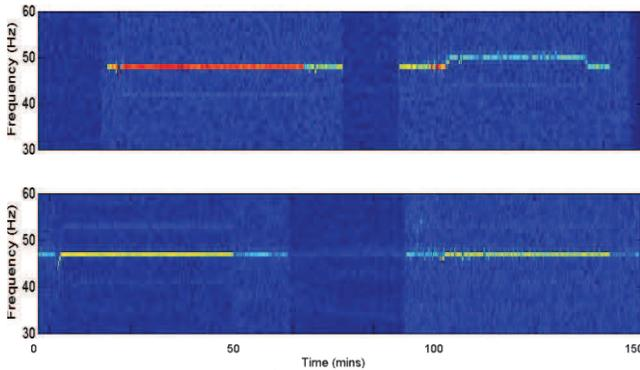
Fig 3: Processed vibration data from two ferries (one return crossing per ferry). Red =  $1000mg_{pk}$
