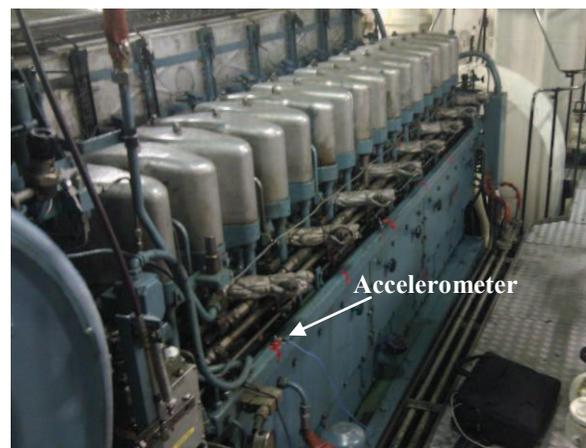
Fig. 2: Eight-cylinder diesel main engine on ferry
