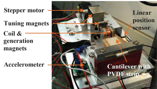
Fig. 7: Assembled generator
