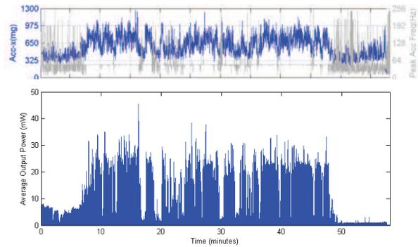
Fig. 10: Results from real test on ferry: power delivered to optimal load, and vibration levels
