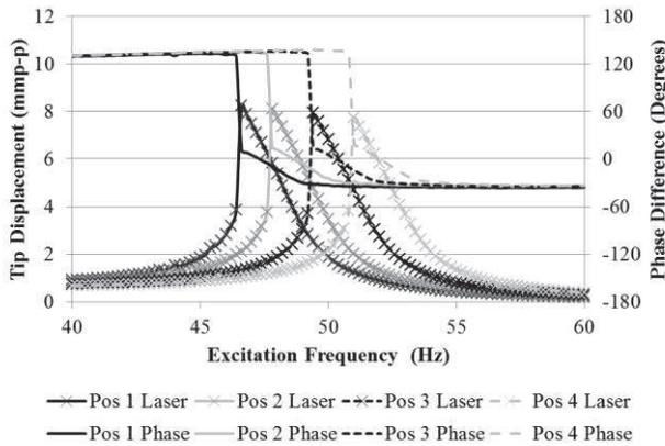
Figure 9: Generator performance with excitation frequency up-sweeping, amplitude  $1000m_{g_{pk}}$
