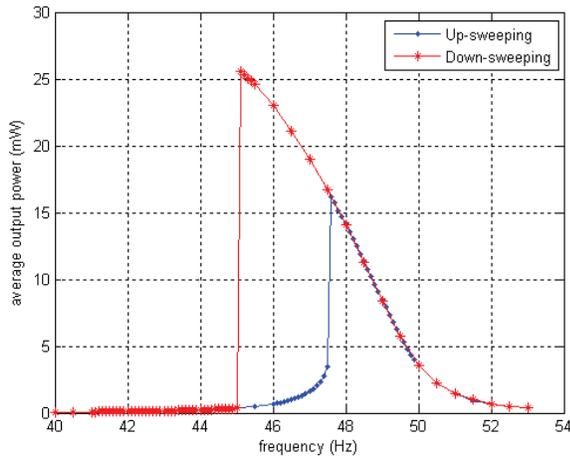
Fig. 8: Average output power when the generator was excited at  $950m_{g_{pk}}$  at 48Hz
