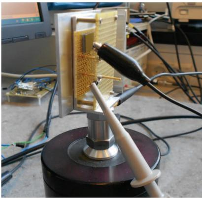
Fig. 6: Device mounted on a piezoelectric shaker with the test circuit connected.
