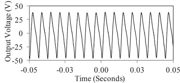
Figure 7. Output voltage on a 20-M $\Omega$  load at 4-g acceleration at 156Hz.
