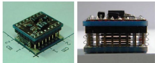
Figure 4. Assembled energy harvesting system.
