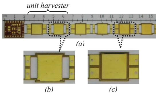
Figure 2. (a) FPCB for device assembly, (b) electret-electrode with low resonance frequency, (c) counter electrode with high resonance frequency.
