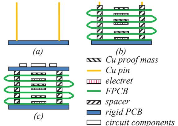
Figure 3. Fabrication and assembly process.
