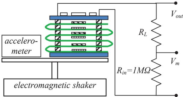
Figure 5. Power generation measurement setup.
