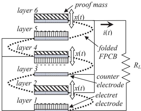
Figure 1. Folded and stacked out-of-plane electret energy harvesters.
