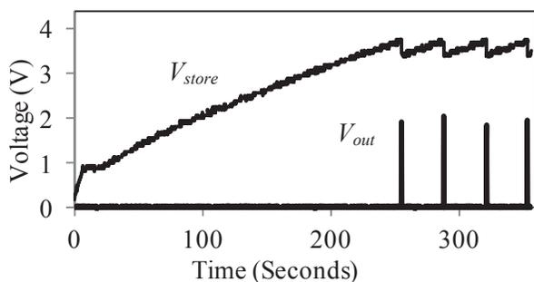
Figure 12. Measured  $V_{store}$  on the storage capacitor and  $V_{out}$  at the output terminal of the power management IC at 4-g acceleration at 156 Hz.
