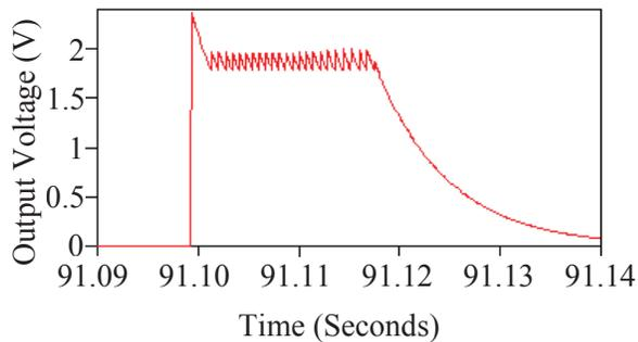
Figure 11. Simulated  $V_{out}$  output burst.
