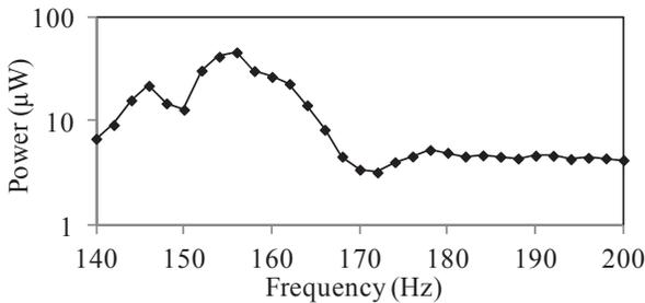
Figure 6. Frequency response on a 20-M $\Omega$  load at 4-g acceleration.
