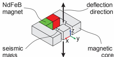
Fig. 1: Basic design of the springs with a cubic mass. The mass is pulled back into the gap upon a deflection along the z-axis. The picture shows the position of zero deflection.
