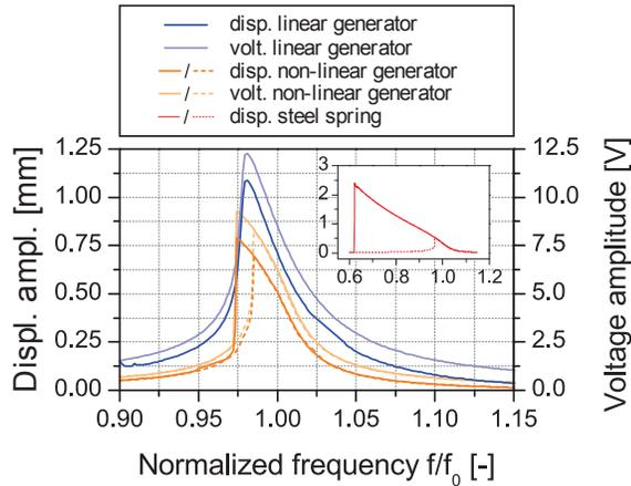
Fig. 7: Measured frequency response (at 5 m/s<sup>2</sup>) for a piezoelectric generator without reluctance spring and with bulk reluctance spring. Frequencies are normalized to the linear resonance frequency for better comparison. The inset shows the frequency response of a steel spring with reluctance spring.
