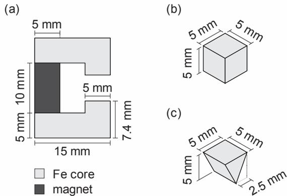
Fig. 2: Dimensions of the fabricated spring design. (a) shows the reluctance circuit with a homogeneous thickness of 5 mm, (b) the cubic mass, and (c) the wedge-shaped mass.
