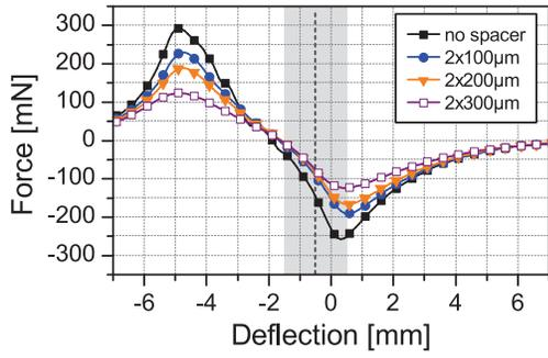
Fig. 4: Measured spring characteristics for different spacer geometries. The indicated range (grey) provides the strongest nonlinearity for the wedge-shaped mass
