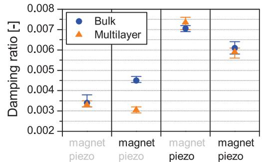
Fig. 6: Measured damping ratio for different combinations of linear and reluctance springs.
