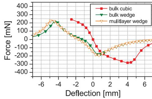
Fig. 3: Measured spring characteristics for different mass geometries and core types.
