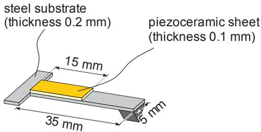
Fig. 5: Piezoelectric unimorph generator with attached wedge-shaped mass.
