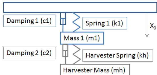
Figure 1: Schematic representation of two mass-two spring setup, where the harvester is connected to an additional mass-spring system.
