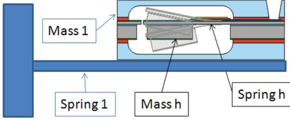
Figure 3. Practical setup of the two mass-spring system. The Energy Harvester has mass  $m_h$ , spring constant  $k_h$ . The mass of the packaged MEMS device (minus the mass of the harvester mass) and beam form mass  $m_1$ , is placed on a metal beam with spring constant  $k_1$ .
