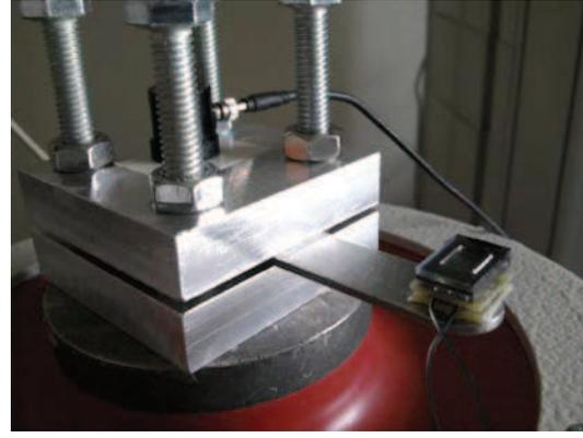
Figure 4: Experimental setup: The packaged MEMS harvester is placed on top a 1mm thick metal beam. The beam is clamped and attached to a shaker. On top of the metal clamping, the accelerometer (black) is visible.
