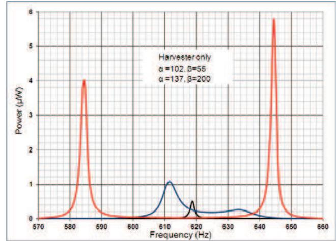
Figure 6. The original harvester power output (black line) compared to the amplified signal (red line). The maximum power is 11.5 times larger than the original maximum ( $\alpha = 102, \beta = 55$ ). An example of bandwidth broadening of the amplified signal (blue curve), by changing  $k_1$  and  $m_1$ , such that  $\alpha = 137$ , and  $\beta = 200$  (ext. input = 0.08g)
