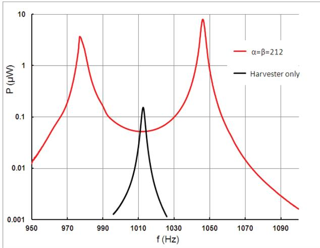
Figure 7: The power output for a PE harvester with  $f_h$  of 1011 Hz (external input= 0.08g). An amplification factor of 51.3 times is obtained ( $\alpha = \beta = 212$ )
