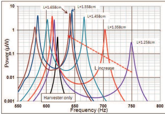
Figure 5. Resonance curves of the coupled system for different lengths  $L$  of the beam. For comparison, the original harvesters signal (black) is included (ext. input = 0.08g)
