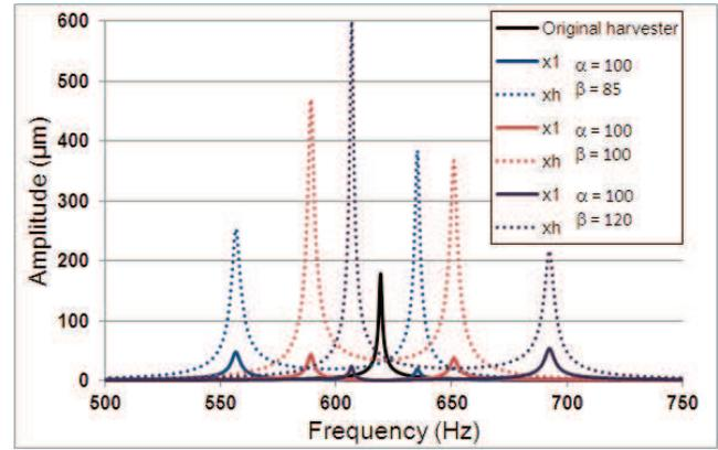
Figure 8. The amplitudes of the harvester ( $x_h$ , dotted lines) and the beam ( $x_1$ ), for  $\alpha=100$  and different  $\beta$  values. For comparison, the amplitude of the original harvester amplitude is plotted (black solid line)
