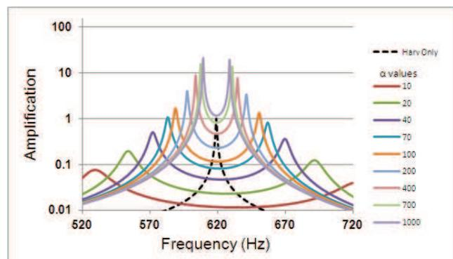
Figure 2: Modeling of the amplification effect. The relative gain of the harvester amplitude is plotted for different values of  $\alpha$  and compared to the original harvester's amplitude (the black curve).
