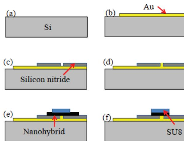
*Fig. 2: Fabrication process flow: (a) Start with p-type silicon wafer; (b) Au pattern is formed on the silicon substrate; (c) Silicon nitride is deposited and then patterned; (d) top Au pattern is formed; (e) CNT-CuS nanohybrid thin film is transferred on the substrate and SU8 layer is patterned; (f) the hybrid nanomaterial thin film is patterned using SU8 as a mask*
