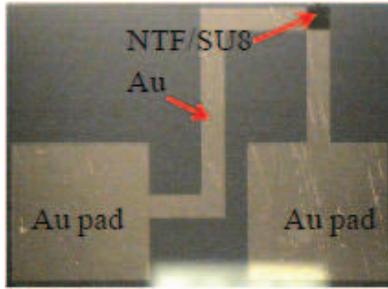
Fig. 4: Photo of a fabricated thermoelectric micro generator. The NTF is integrated in the Junction I region
