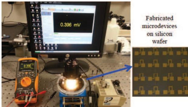
Fig. 5: The experimental setup for the measurements of voltages and currents by the thermoelectric microgenerators
