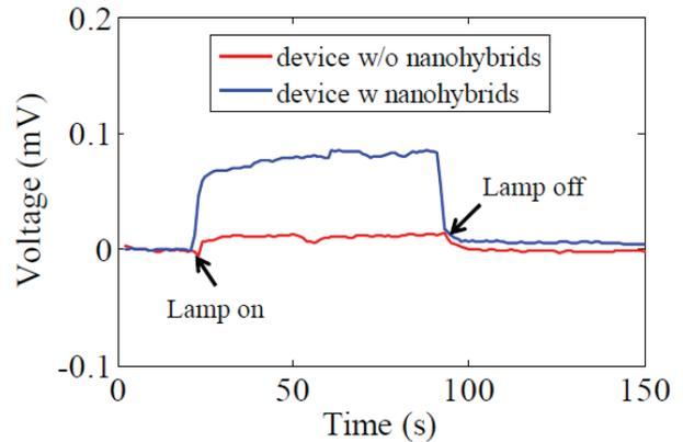
Fig. 6: Measured open circuit voltage (OCV) of a thermoelectric microgenerator with and without Nanohybrids (NTF) under uniform lamp illumination
