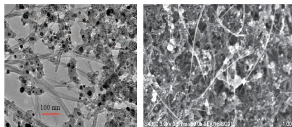
*Fig. 3: (left) the TEM image of CNT-CuS NPs hybrid nanomaterial; (right) the SEM image of the CNT CuS NPs thin film*
