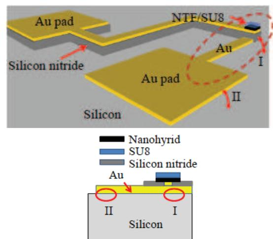
*Fig. 1: Sketch of a thermoelectric microgenerator with integrated NTF:(left) angled topside view; (right) cross-section showing the junction I and II formed between silicon substrate and Au layer*
