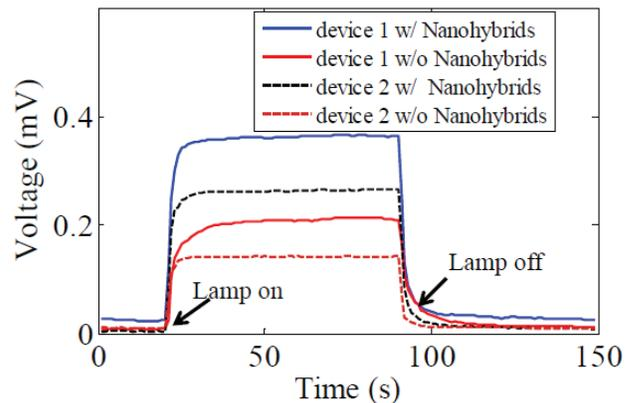
Fig. 7: Measured open circuit voltage (OCV) when the lamp illumination is only on the Nanohybrids(NTF) region compared to a device without the integrated Nanohybrids (NTF)
