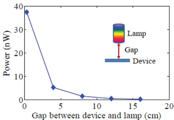
Fig. 8: Measured peak power by the thermoelectric microgenerator under different light intensity and temperature of the lamp by changing the gap between the device and the lamp
