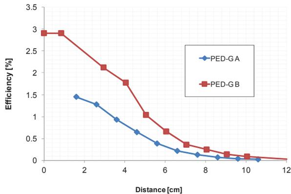
Fig. 6: The efficiency vs. distance of the far-coil setup for PED-G prototype A (blue) and B (red) operating in the torque mode.
