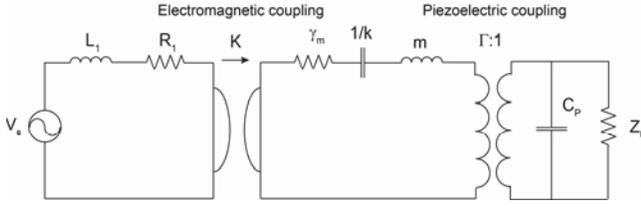
Fig. 2: Lumped-parameter circuit representation of a PED-G.
