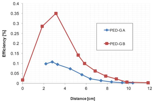
Fig. 5: The efficiency vs. distance of the far-coil setup for PED-G prototype A (blue) and B (red) operating in the force mode.
