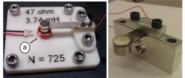
Fig. 3: PED-G prototypes A (left) and B (right). Prototype A is shown attached to the near-coil transmitter (a).
