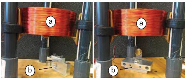
Fig. 4: Far-coil experimental setup for PED-G prototype B in force (left) and torque (right) configurations.
