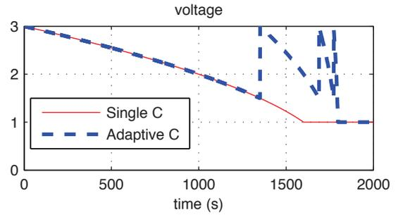
Fig. 3: evolution of discharge voltage vs. time ( $V_{min}=1V$ )
