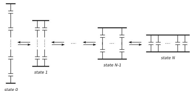
Fig. 1: successive arrangements of elementary capacitors, from the smallest equivalent value (state 0) to the maximum equivalent capacitance (state N).
