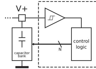
Fig. 7: block schematic of the control circuit
