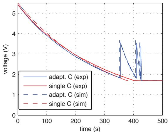
Fig. 9: Discharge voltage for a fixed capacitor (a) and an adaptive capacitor (b)
