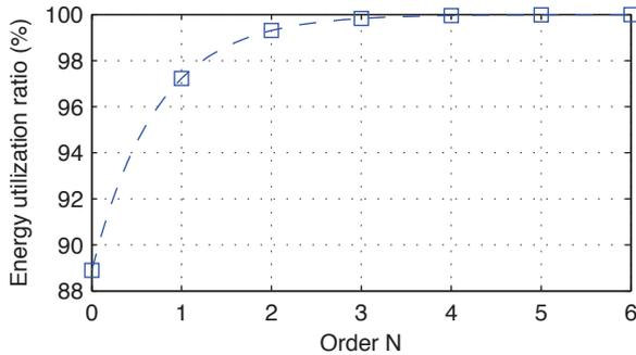
Fig. 5: Energy utilization ratio vs. order  $N$ , according to equation 2 (assuming  $V_{\text{min}}/V_{\text{max}}=1/3$ ).
