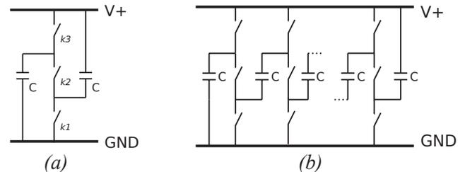
Fig. 4: schematic of the basic cell (a) and the generic architecture (b)
