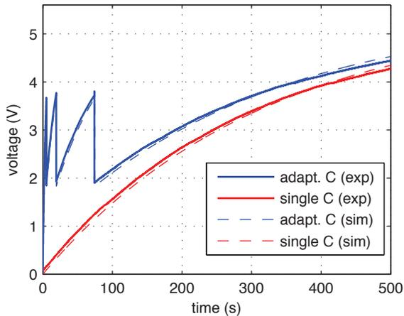
Fig. 8: Charge voltage for a fixed capacitor (a) and an adaptive capacitor (b)
