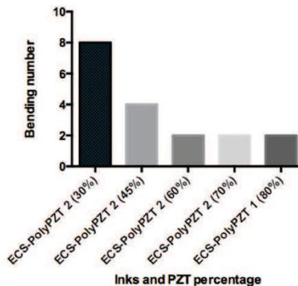
Fig. 5: Number (cycles) of complete bending test
