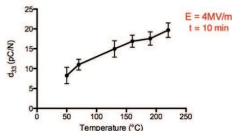
Fig. 7: Poling temperature optimization
