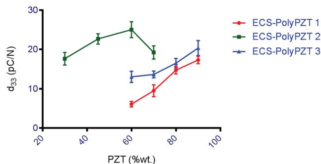
Fig. 4: Piezoelectric coefficients versus percentage of PZT by weight in the composites. Poling parameters were taken at fixed conditions ( $E = 6 \text{ MV/m}$ ,  $T = 160 \text{ }^\circ\text{C}$  and  $t = 10 \text{ min}$ )
