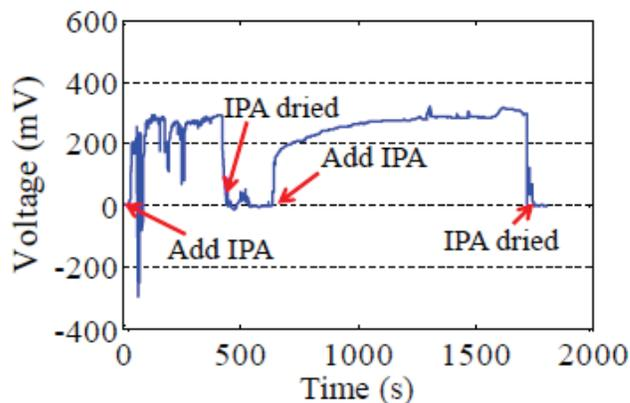
*Fig. 4: Measured open circuit voltage (OCV) of a CNF device when the IPA solution was applied. It was found that when the PIA dried, the voltage became essentially zero. By adding IPA, the voltage can be recovered*
