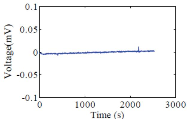
*Fig. 3: Control experiments on a CNF device without applying any liquids: Measured open circuit voltage is essentially zero*
