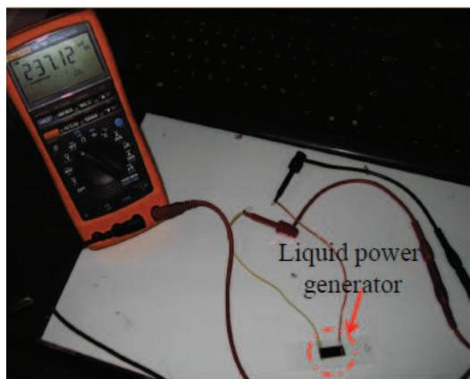
*Fig. 2: Photo for the typical experiment setup to measure the open circuit voltage and power generation*
