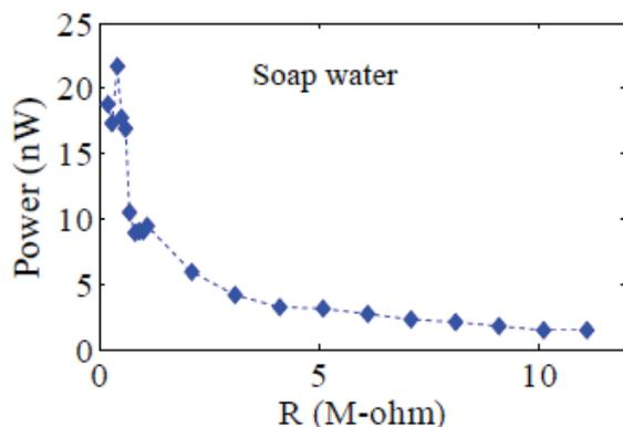
Fig. 6: Measured power generation of the CNF device when soap water was applied by changing the loading resistance
