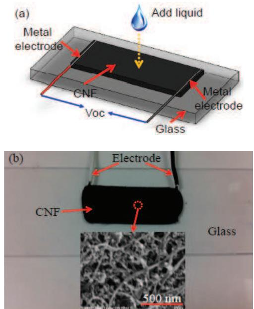
Fig. 1: (a) Sketch of the CNF-based device; (b) Photo of a fabricated CNF device; Inset is the SEM image of the CNF. The thin-film device measures 2 cm long, 0.8 cm wide and 100  $\mu\text{m}$  thick
