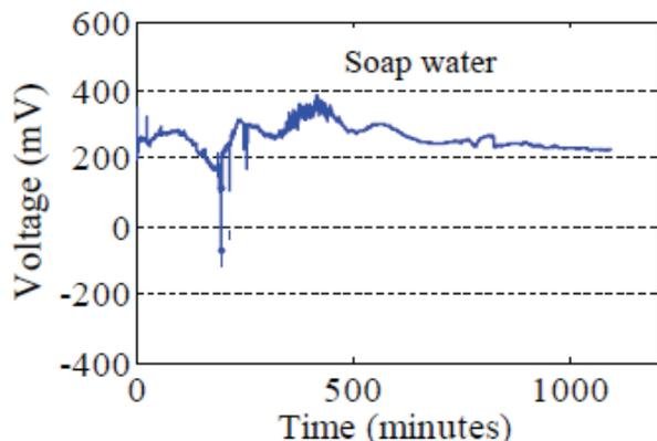
Fig. 5: Measured open circuit voltage (OCV) of a CNF device when soap water was applied
