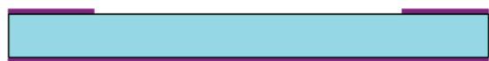
(a) Photolithography of top resist to define the basins. Protect bottom from etching.
