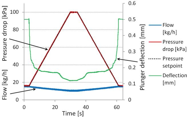
Fig. 5: Closed-loop pressure control: linearly increasing and decreasing pressure input.
