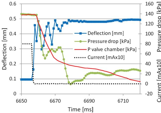
Fig. 4: Response time at valve opening.
