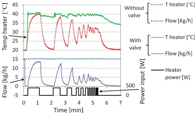
Fig. 10: Closed-loop temperature control vs. a system without control valve: sudden heat load.
