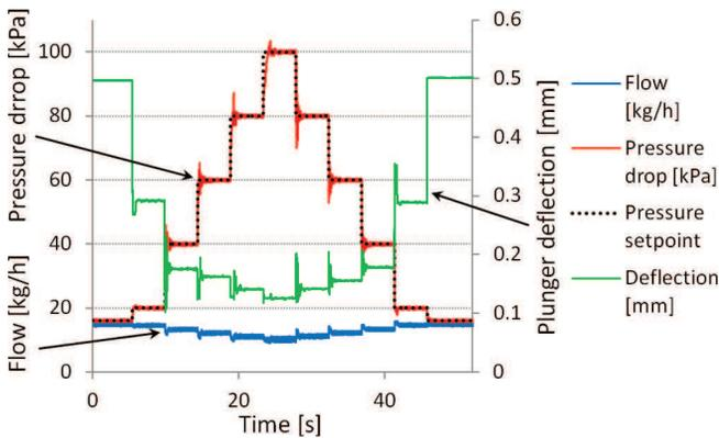
Fig. 6: Closed-loop pressure control: stepped increasing and decreasing pressure input.
