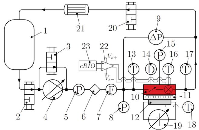
Fig. 3: Schematic representation of the measurement system.
