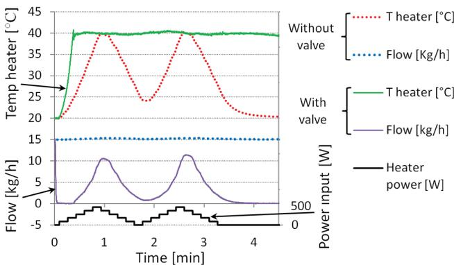
Fig. 9: Closed-loop temperature control vs. a system without control valve: gradual heat load.
