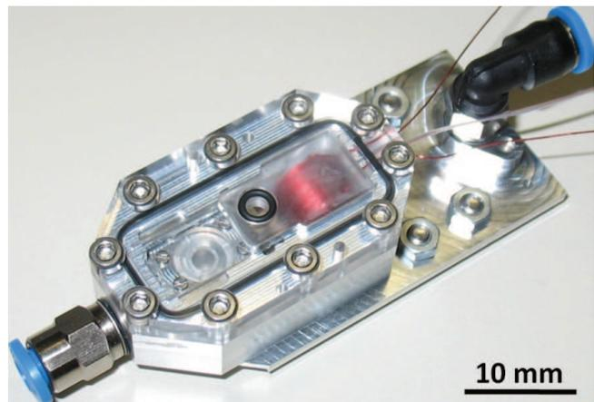
Fig. 1: Assembled electromagnetic valve on the heat sink.
