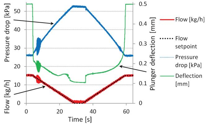
Fig. 7: Closed-loop flow control: linearly increasing and decreasing flow.
