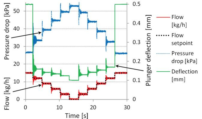
Fig. 8: Closed-loop flow control: stepped increasing and decreasing flow.
