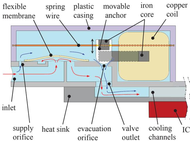
Fig. 2: Schematic of the valve operating principle.
