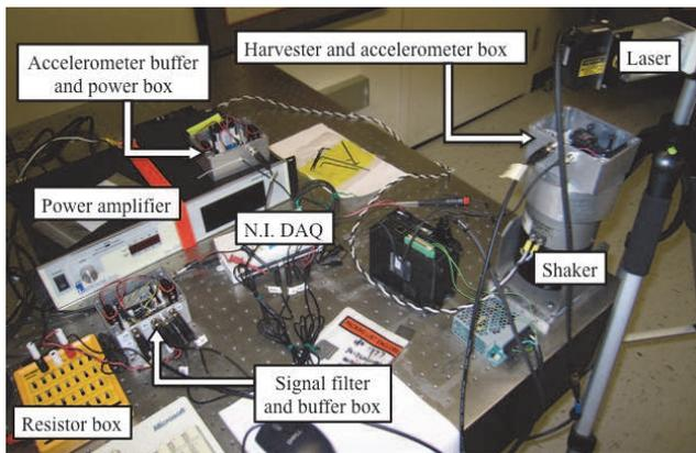
Fig. 4: Vibration platform components
