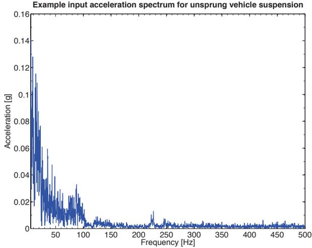
Fig. 2: Representative acceleration spectrum for the unsprung suspension of a passenger vehicle
