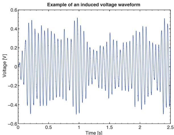
Fig. 5: Induced voltage waveform representative of the mean power harvested in the 97+ kph category of the trip from San Mateo to Berkeley.
