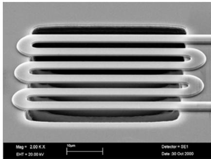
**Figure 8.** 50  $\mu\text{m}$  sq. flow/rpm sensor.
