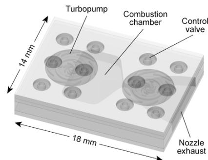
**Figure 1.** Micro-bipropellant MEMS rocket engine concept sized for 10-15N thrust.
