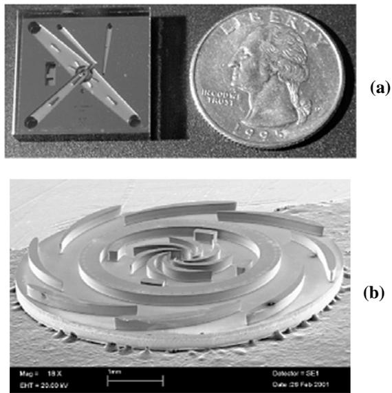
**Figure 6.** Demonstration microturbopump: a) 2 cm sq turbopump chip; b) 6 mm dia turbopump rotor.
