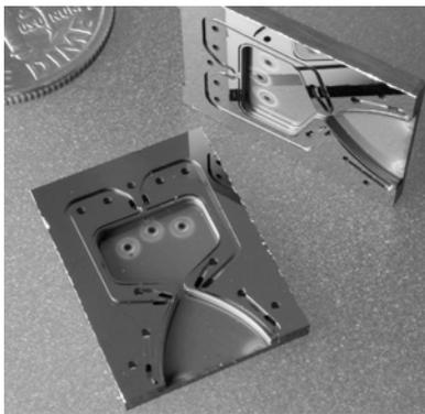
**Figure 3.** Cooled Si combustion chamber-nozzle.
