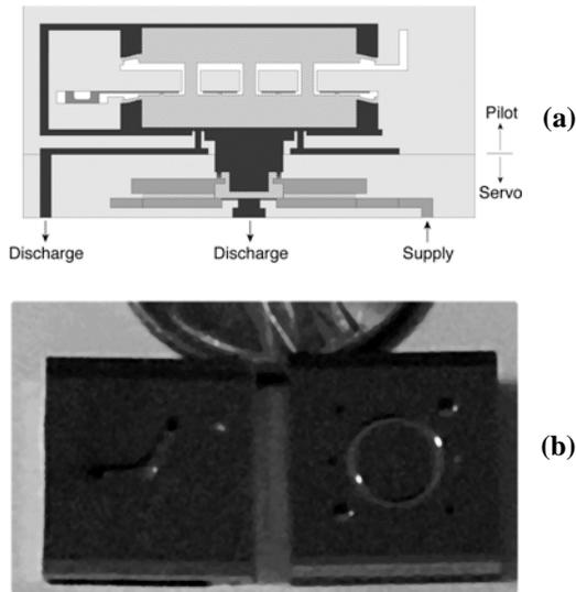
**Figure 7.** Rocket propellant valve: a) valve cross-section, b) valve prototypes, servo (left) & pilot (right).
