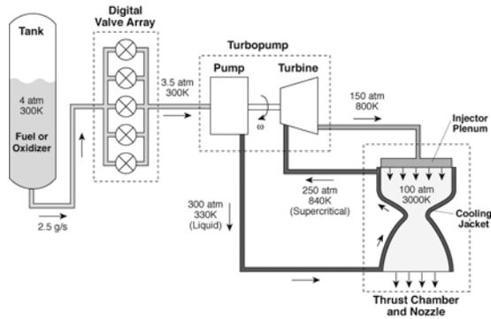
**Figure 2.** Evaporator cycle, pump-fed microrocket engine system.
