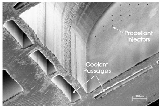
**Figure 5.** Cutaway TCA head showing cooling passages and propellant injectors.
