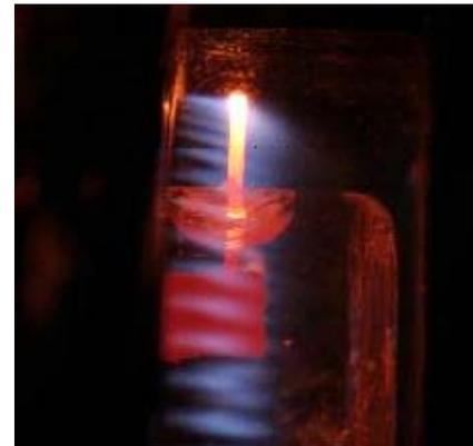
Figure 6 - Combustion test in the quartz chamber at design point  $\lambda=6$  and air mass flow of 6.7 g/s
