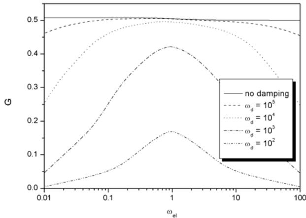
Fig. 3: Figure of merit  $G$  in dependence on  $\omega_{el}$  and  $\omega_{dl}$  for a structurally damped converter with  $k = 0.1$ .
