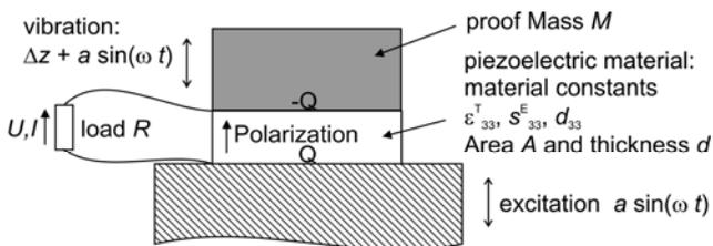
Fig. 1: Model representation of a piezoelectric energy harvester.
