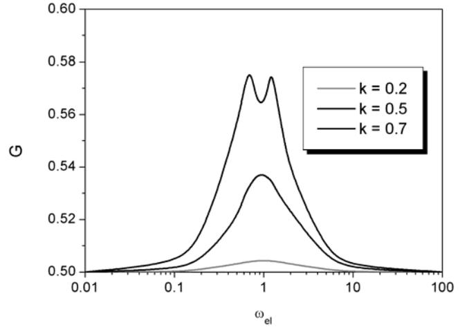
Fig. 2: Figure of merit  $G$  for an idealized converter in dependence on the electrical damping frequency  $\omega_{el}$ .
