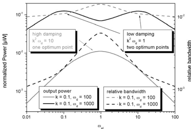
Fig. 4: Power and bandwidth for a real harvester with high and low structural damping.
