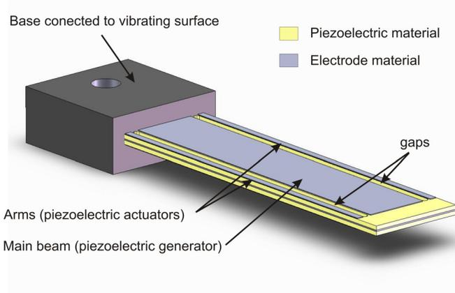
Fig. 3: Generator with arms made out of one dual layer piezoelectric plate.
