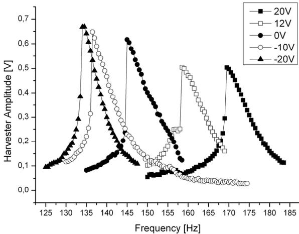
Fig. 8: Resonance curves for device 2 at different positive and negative actuator voltages.
