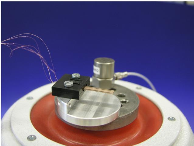
Fig. 5: Experimental Setup. The harvester is clamped to a shaker performing sinusoidal oscillations. In the background, an accelerometer can be seen.
