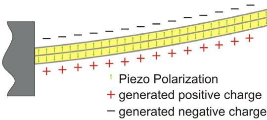
Fig. 1: Piezogenerator (main beam).
