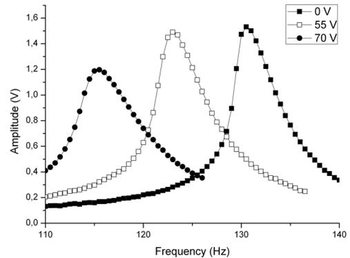
Fig. 6: Resonance curves of device 1 for a positive actuation voltage.
