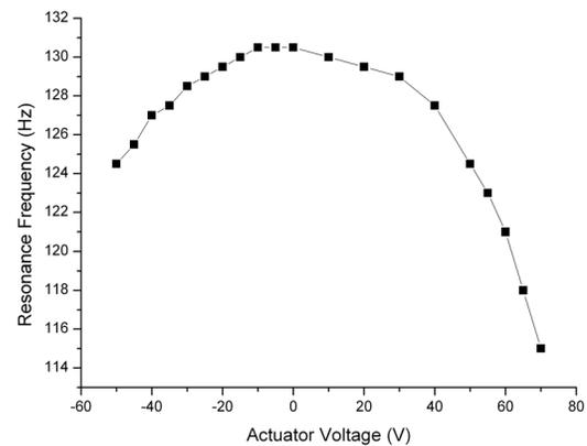
Fig. 7: Frequency shift of device 1 for positive and negative actuation voltages.
