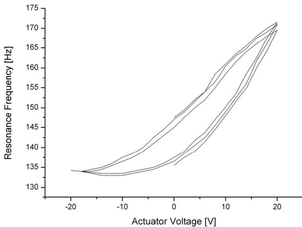
Fig. 9: Hysteresis Curve of device 2 at a voltage range from -20 to 20V.
