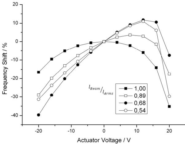
Fig. 4: Simulation Results: With a main beam shorter than the lateral arms, the frequency tuning effect can be enhanced and a larger frequency tuning gradient at low voltages is achieved. For a better comparability, percentaged frequency shifts are displayed.
