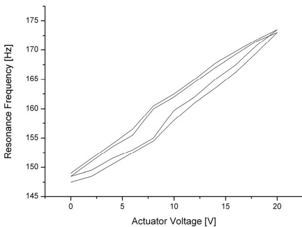
Fig. 10: Hysteresis Curve of device 2 at a voltage range from 0 to 20 V.
