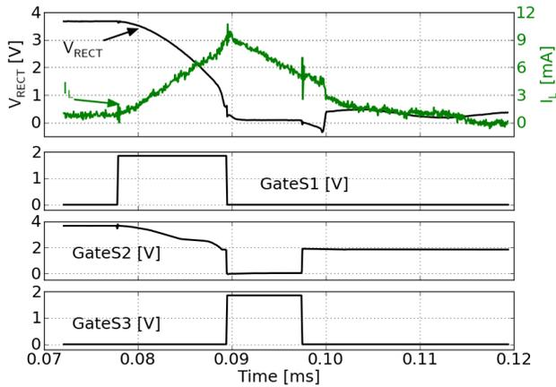
Fig. 6: Measured rectified generator voltage  $V_{RECT}$  and coil current  $I_L$  (top) and gate signals (bottom) of the switches during a transfer process.
