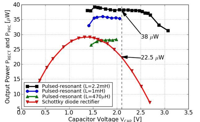
Fig. 5: Measured output power using a Schottky diode bridge rectifier and the pulsed-resonance converter with different coils. The dashed line denotes the operating point using the demonstrator board.
