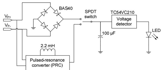
Fig. 3: Schematic of the demonstrator PCB. Via a switch, either the diode rectifier or the PRC can be used as an interface for the piezoelectric generator.
