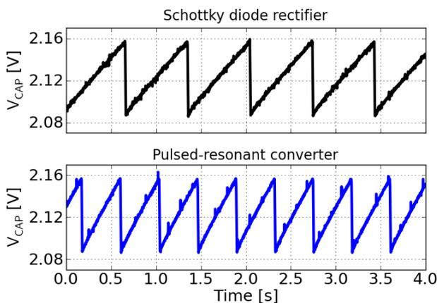
Fig. 7: Capacitor charging and discharging cycles using diode rectifier (top) and pulsed-resonance converter (bottom). The higher the frequency, the more efficient the conversion.
