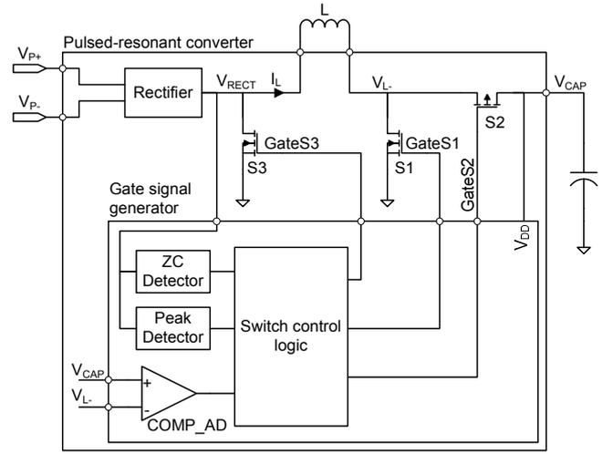
Fig. 2: Block diagram of the pulsed-resonant converter ASIC. The piezoelectric generator is not shown.
