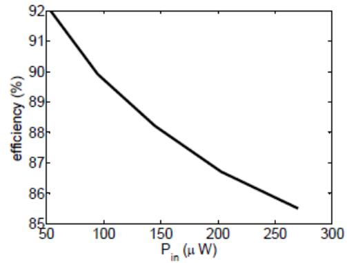
Fig. 7: The efficiency of the power converter versus the input power.
