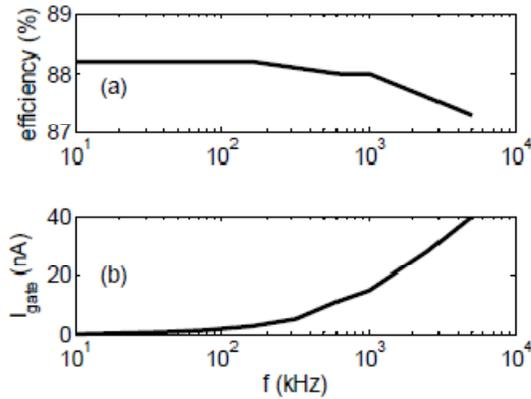
Fig. 6: (a) The efficiency of the power converter versus switching frequency; (b) The gate current versus frequency at duty-cycle  $D=10\%$ .
