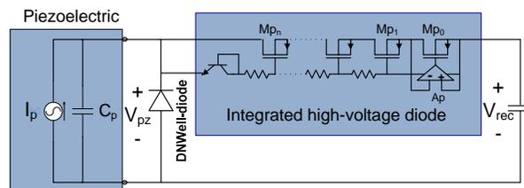
Fig. 2: High-voltage topology for voltage doubler
