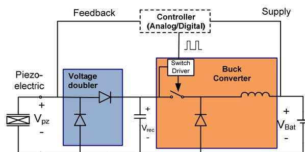
Fig. 1: Schematic diagram of energy harvester circuit
