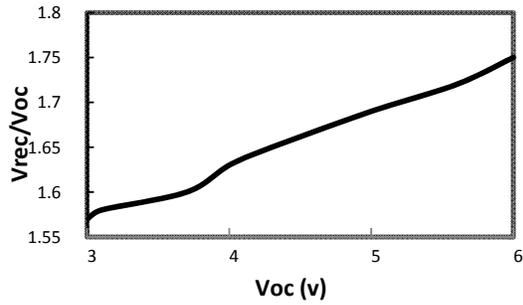
Fig. 5: The normalized rectified voltage ( $V_{rec}/V_{oc}$ ) versus  $V_{oc}$ .
