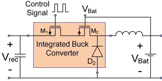
Fig. 3: Schematic of high voltage buck converter
